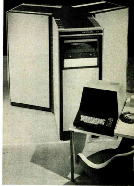
Emulator. Architecture of computer designed by Nanodata can be changed in milliseconds with new type of program control.
