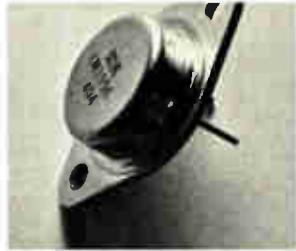
The first transistors that are blow out proof and short circuit proof.
