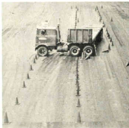
Straight and narrow. Truck at left skids and jackknifes when entering lane on wet pavement. But equipped with electronic antiskid controls, truck at right stays within the 12-foot lane.
