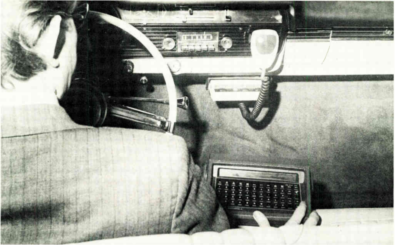
Calling all cars. Microprocessor in Atlantic City, N. J., police station controls message-coding for keyboard terminals used in squad cars.
