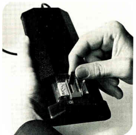
New plug-in reference board sets up quickly and economically for infrequently used ICs.
