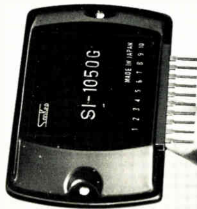
Sanken series SI-1000G HYBRID POWER AMP SI-1010G (10W), SI-1020G (20W) SI-1030G (30W), SI-1050G (50W)
