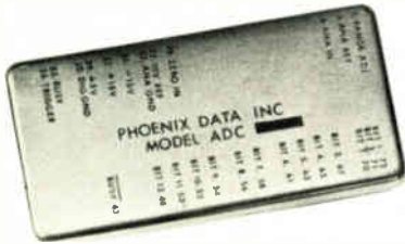
One of two compact cases (2"x4"x.39") that contain the 42 new Phoenix Data modules.
