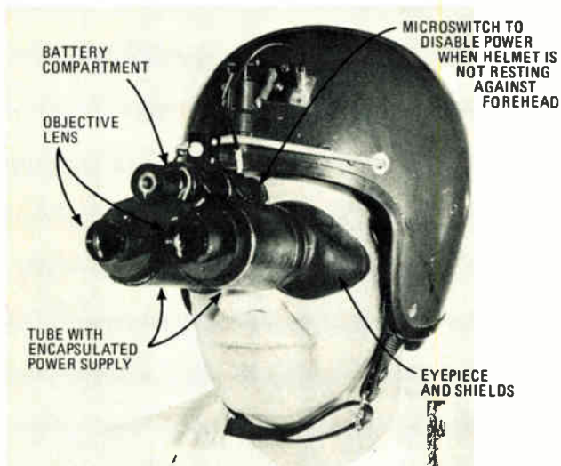
6. Night driver. Night-viewing binoculars developed at Mullard are an example of the new applications made possible by the reduced size of microchannel-plate intensifiers. The helmet-mounted microchannel unit shown, which includes batteries and necessary optical lenses, enables scenes to be viewed easily even in starlight.
