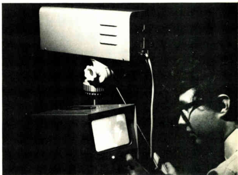
8. Surveillance monitor. Image on cathode-ray-tube display is produced by system in which microchannel inverter tube is coupled to vidicon camera. Target, which is 25 meters away, is illuminated only by the stray light that was used to take this picture (i.e., conditions which are an approximation of starlight).
