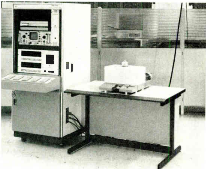
Tester. Computest "Venture" semiconductor-memory tester includes storage file, scope, error display, and keyboard (left).
