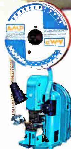
AMP-O-MATIC stripper/crimper machine strips wire and attaches contact during each machine cycle—at rates up to 1500 an hour.
