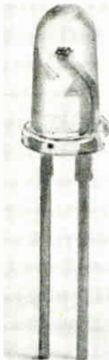
CM4-20 GaAsP, clear transparent lens, intense point source indicator.
