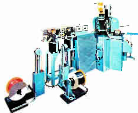
AMPOMATOR machine with miniature applicator can produce up to 5700 doubly-terminated leads an hour.
