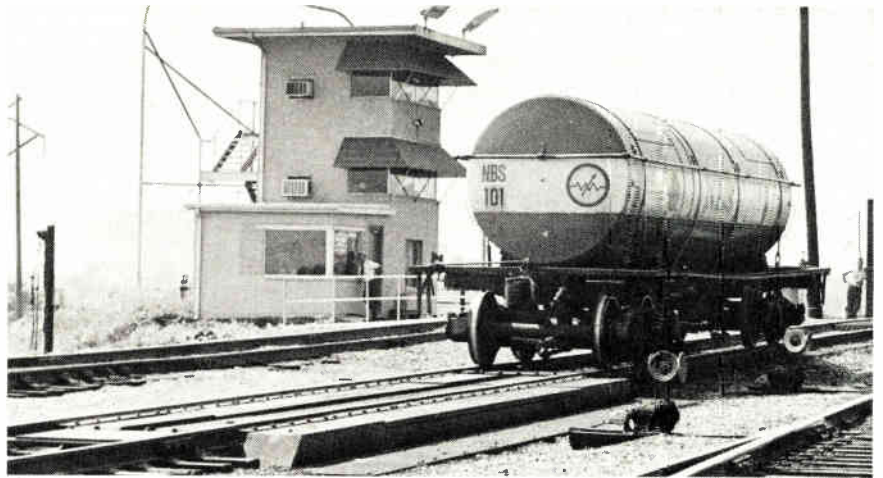
Humped. National Bureau of Standards test car approaches 20-ft. section of track where electronic scale weighs it in Alexandria, Va., railroad hump yard.
