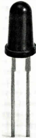
CM4-23 GaAsP, red translucent lens, diffused light source.
