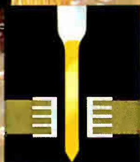
Presoldered contact is inserted into plated panel through-hole.
