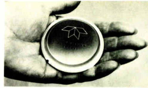
Handful. Teledyne Systems' microcomputer is 2.5 in. in diameter and sells for $1,000.
