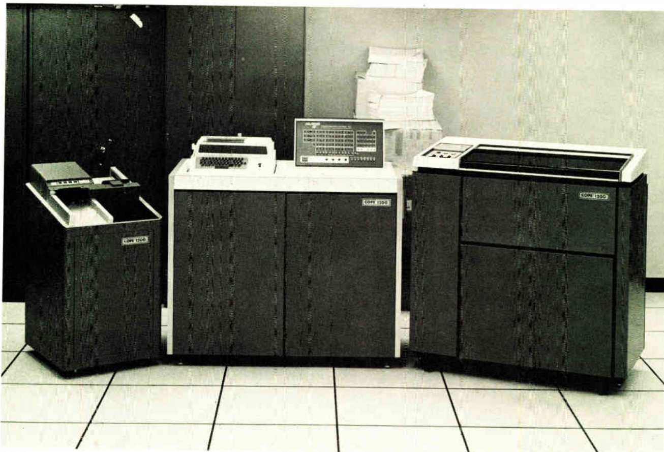
Intelligent terminal. Minicomputer-based terminal controller (center) provides code conversion, error correction, and even limited local processing for a cluster of terminals remote from the host computer. Any of a number of terminal units can be attached to the controller, such as the 300-card-per-minute card reader (left) and the 600-line-per-minute printer (right) marketed by Harris Communications Systems.
