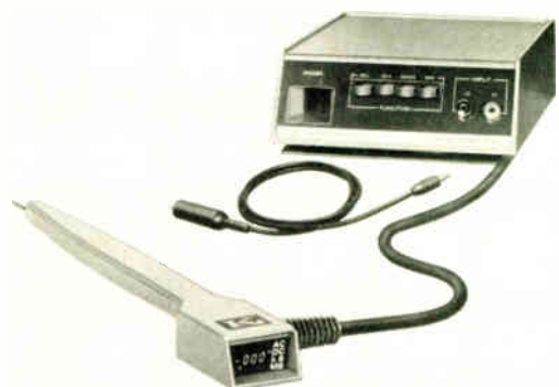
5. Proven performance. Charge-balancing converter is heart of this portable multimeter. Extensive field experience proves that new conversion technique is worth considering for new system designs.
