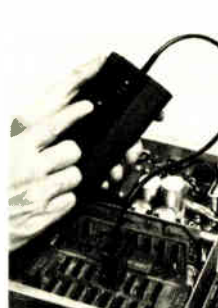
Attach the clip to the suspect IC and check the comparator display.
