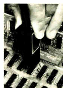
The suspect and reference IC are compared automatically. Indicator lights signal which pins are faulty.
