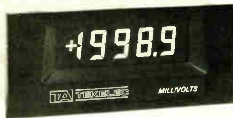
10. Power saver. This Tekelec digital panel meter uses a field-effect liquid-crystal display. Although it requires backlighting, it only needs a 0.5-watt bulb to obtain an excellent contrast ratio.
