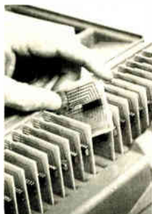
Select a reference board with a good IC that has the same type number.
