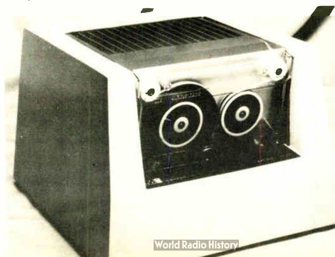
Compact. Mohawk desktop tape handler uses 3M cartridge.
