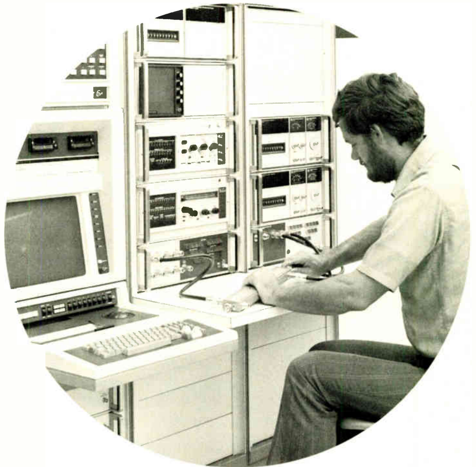
Shown here testing a UHF component, the HP 8580B serves as a cost-effective production test station.
