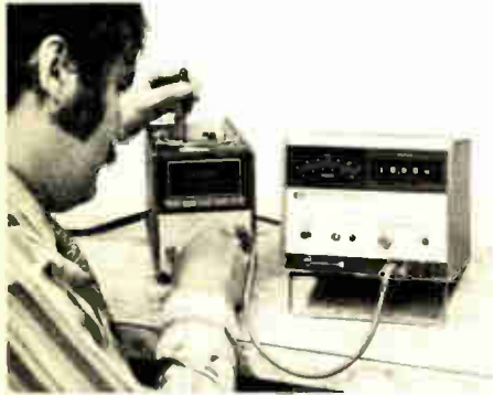
A 6115A precision power supply is used to calibrate the dc voltmeter section of an HP multimeter.
