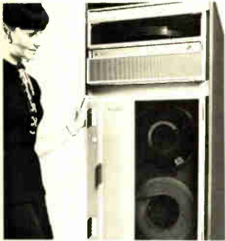
The 7900 disc drive (top) and 7970 tape transport (underneath) are compact, flexible peripheral memories.
