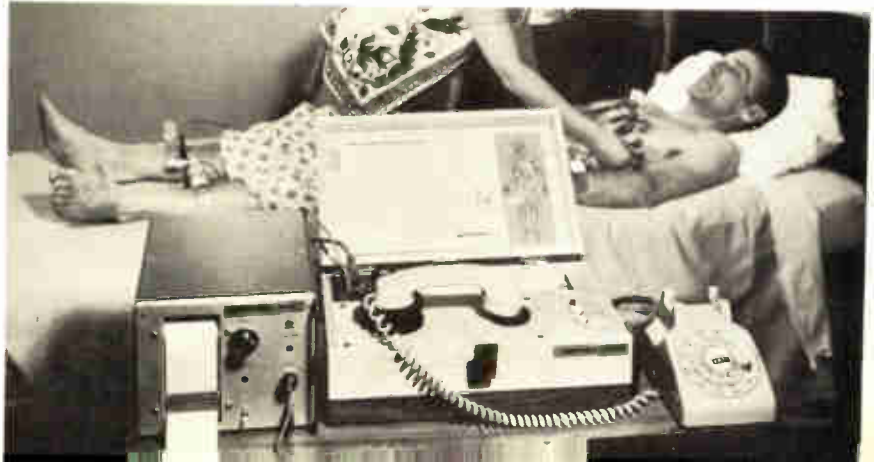
Remote. Phone-a-gram EKG reader promises lower cost, faster service from bedside.
