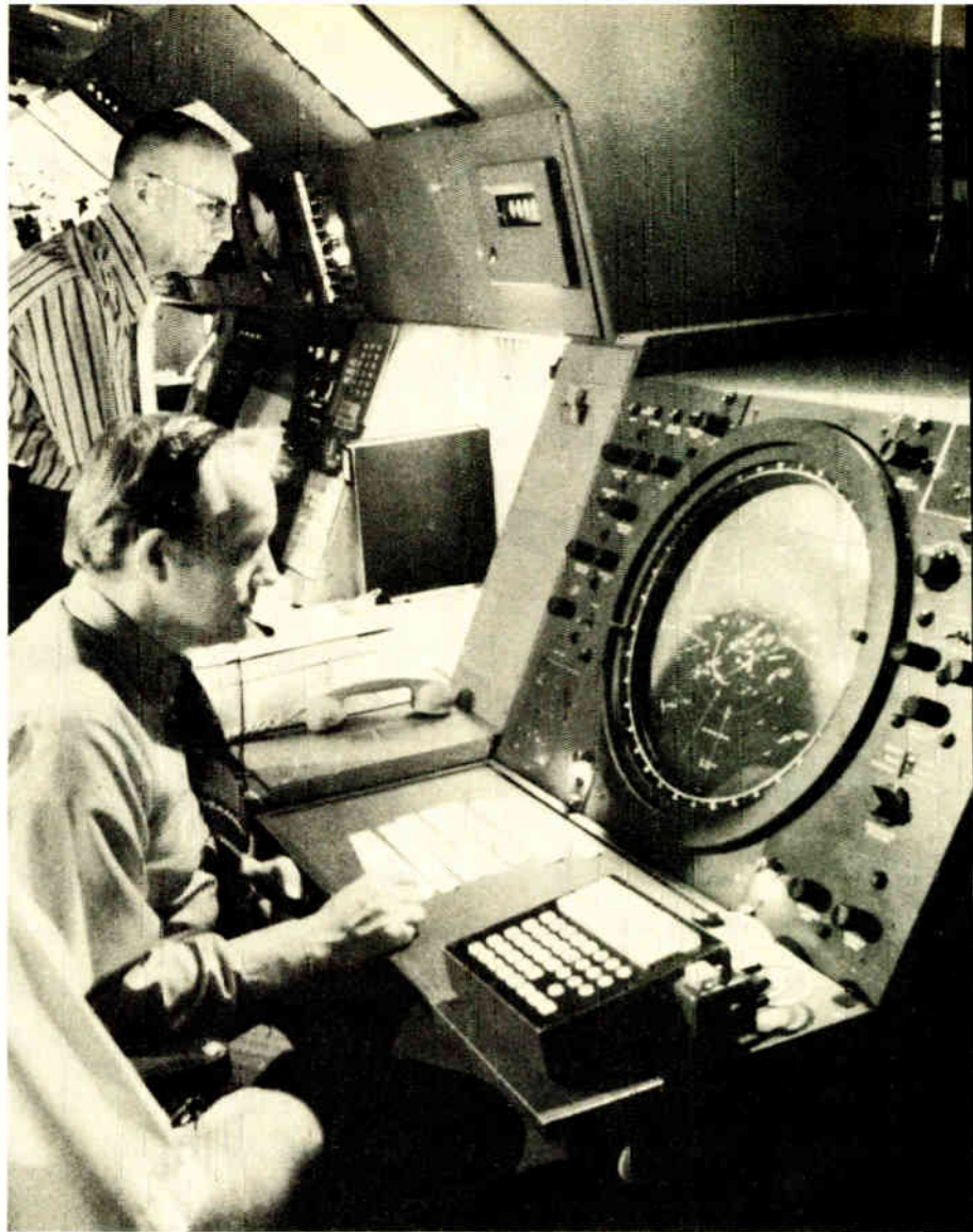
Airy predictions. When the Staran associative processor is tied in with air traffic control radar, it can predict aircraft paths and determine if any aircraft are on collision courses.
