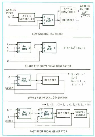
7. Other applications. Principal applications of new multiplier are in digital function generators, fast Fourier transform processors, and arithmetic function generators, which will be able to use configurations like these to expand their capabilities.
