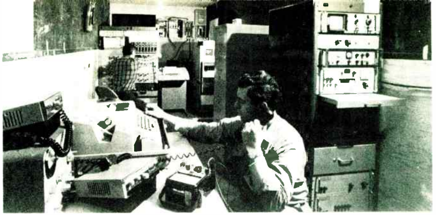
Rescue and survival. Westinghouse electromagnetic communications surface equipment helps locate trapped miners who contact it through a belt-worn low-frequency transmitter.
