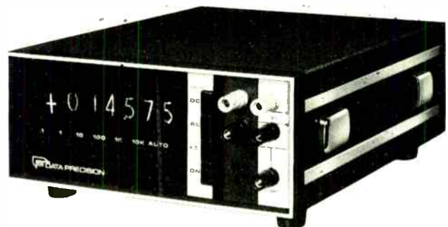
Model 2540. 5½ digits. DC volts, AC volts, Resistance, Voltage Ratio. Auto-ranging. Auto-Polarity. Isolated BCD outputs. Remote triggering. Remote ranging. Basic accuracy ±0.001% f.s. ±0.007% rdg ±1 l.s.d. for 6 months. One-piece price: $1,195.00
