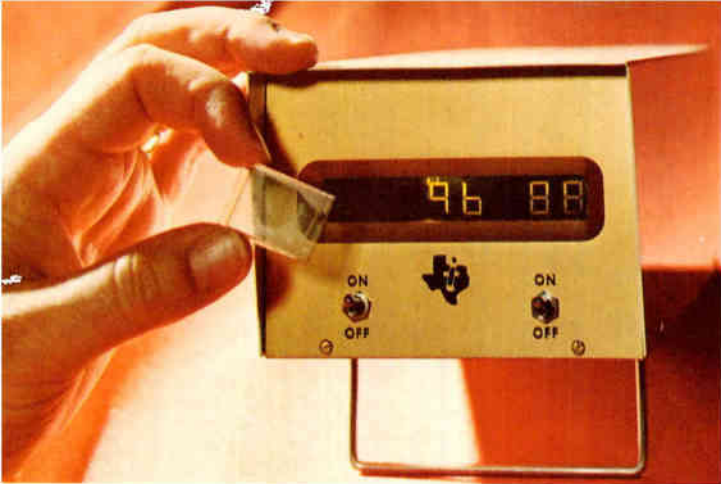
3. Liquid crystals in place. Convinced that lifetime limitations and other problems can be solved, several major firms already are thinking of applications for their liquid crystal readouts. At left is multimeter put together at Texas Instruments. At right is calculator fitted with liquid crystal display made by France's Thomson-CSF.
