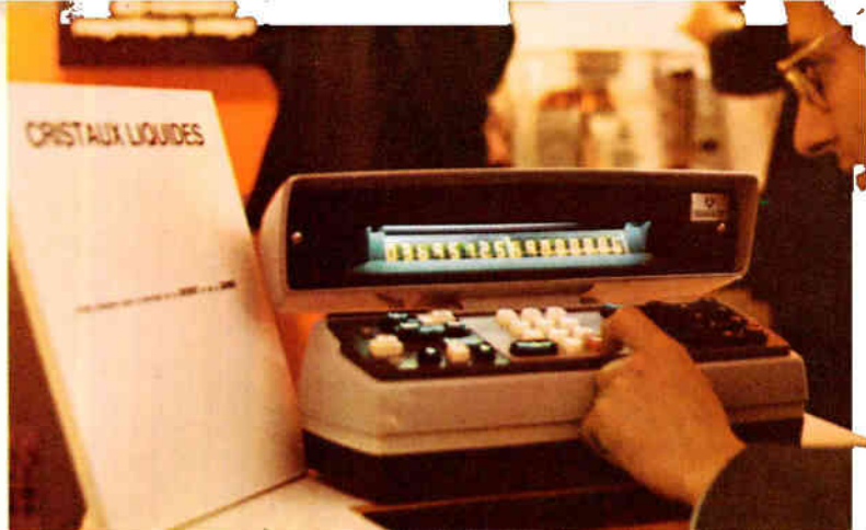
3. Liquid crystals in place. Convinced that lifetime limitations and other problems can be solved, several major firms already are thinking of applications for their liquid crystal readouts. At left is multimeter put together at Texas Instruments. At right is calculator fitted with liquid crystal display made by France's Thomson-CSF.
