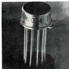
Hybrid ICs DH0034/34c handle voltage level translations among peripherals, data transmission systems and memory devices on two channels at a time. Typical propagation delays are 15 ns to a 0 and 35 ns to a 1. Prices are $11.20 to $26. National Semiconductor Corp., Semiconductor Dr., Santa Clara, Calif. [440]
