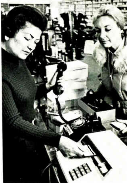
Cash call. IBM's credit authorization terminal uses acoustic coupler attached to telephone's mouthpiece.
