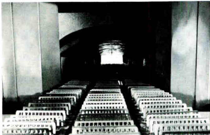
Sealing cerdip at 550° C
