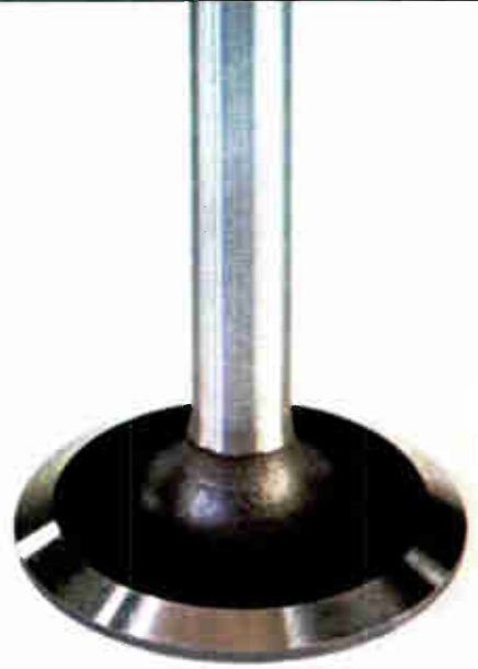
Checking surface geometry of valve section to ensure proper seating.
