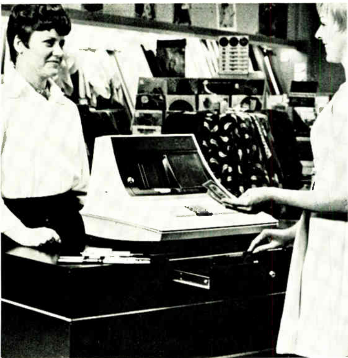
5. Store's store. Friden's Modular Data Transmission System (MDTS) terminal uses a continuous tape loop in a $650 module for daily transactions to the data processing center for updating inventory, recording charge purchases, and initiating reorders.
