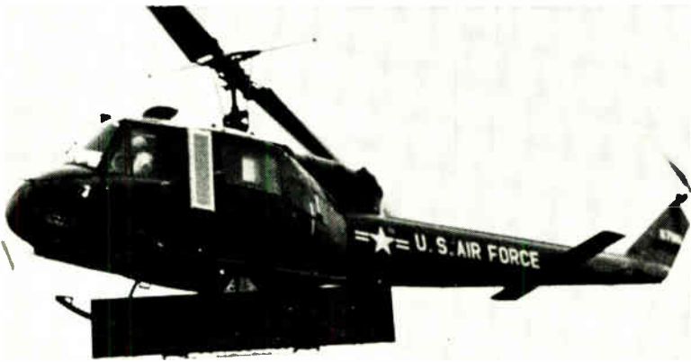
Hanging in. Radar antenna—a corporate-fed planar array of pc dipoles—for system with data-remoting capability stows between copter's skids.
