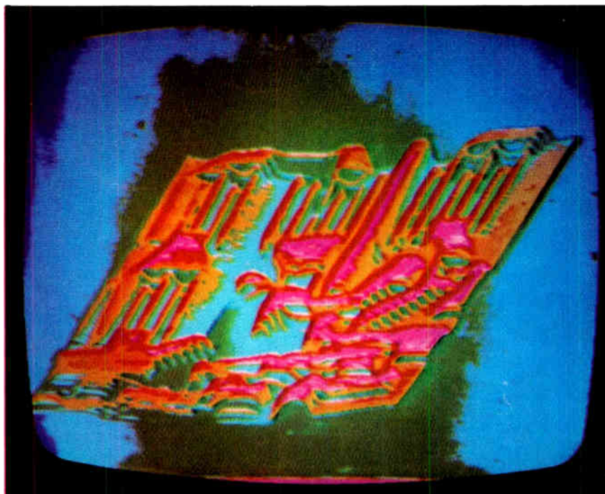
Hot spots on display. Red areas show where current flow is overheating a thin-film hybrid amplifier when test voltages are applied. To get color thermograms on the CRT screen, a converter is required.
