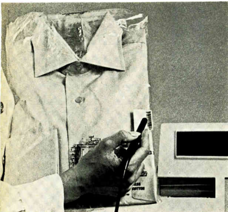
4. Optical reading. The NCR 785 reader picks up optically encoded series of white, black, and green bands containing 10 characters per inch. It's connected to a 280 point-of-sale stand-alone register. Instructions above keyboard tell clerk how to enter information.
