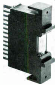
Plug-in modules series DM-17G are factory-assembled, ready-to-use devices featuring a miniature Elfin display and decoder-driver. The neon Elfin is front mounted on a pc board that contains the decoder-driver and the logic required to accept 4-line BCD inputs. All input-output contacts appear on the pc connector. Alco Electronic Products Inc., Box 1348, Lawrence, Mass. [383]
