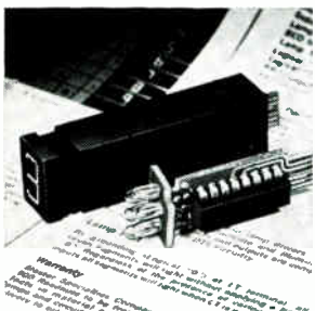
Fiber-optic readout model 901 D2-D8, available with a choice of five different built-in decoder/driver ICs, reduces mounting, wiring and pc board requirements as well as equipment size. The IC decoder and lamp drivers will accept 4 line 8-4-2-1 BCD inputs, translate them and then illuminate proper readout segments. Master Specialties Co., 1640 Monrovia, Costa Mesa, Calif. [385]
