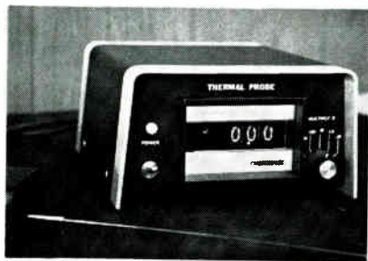
Place and show. A single optical fiber detects infrared radiation which is then displayed as a dc voltage.
