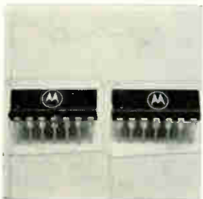
Five dual line driver/receivers, MC1580L-1584L, handle driving/receiving chores in both saturating (MRTL, MDTL, and MTTL) and nonsaturating (MECL) logic systems plus the interfacing between different levels in a system. Units feature high input and/or output impedances in the 5 to 12 kilohms range at 10 Mhz. Motorola Semiconductor Products Inc., Phoenix 85036 [441]
