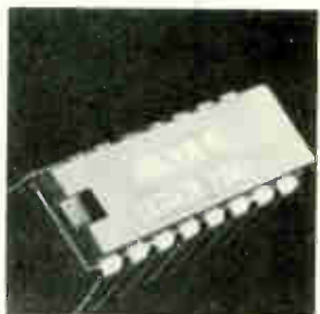
Four-bit binary full adder DM-7283 uses internal carry look-ahead circuitry that cuts ripple time to 12 nsec. Unit is the equivalent of about 30 gates. It accepts four A and four B inputs plus the carry input, and has four sum outputs plus the carry output. It can also be used as a dual single-bit full adder. National Semiconductor Corp., Santa Clara, Calif. [442]
