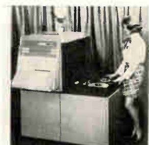
Electronic hard copy terminal model 911 produces page copies of computer graphics in seconds, either on or off line. It is easy to use, featuring pushbutton operation, dry copy, continuous line plots, alphanumeric printing in any size or angular orientation. Approximate price, on-line, is $22,000; off-line, $32,000. Electronic Associates Inc., West Long Branch, N.J. 07740 [388]
