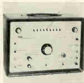
Tv Sweep Chanalyst WR-514A has the combined features of a tv sweep generator, marker generator, marker adder, and special "ChromAlign" system for color bandpass alignment. It provides r-f, i-f, and video output sweep signals for alignment of vhf tuners, i-f amplifiers, video amplifiers, and color bandpass amplifiers. RCA Electronic Components, Harrison, N.J. 07029 [362]
