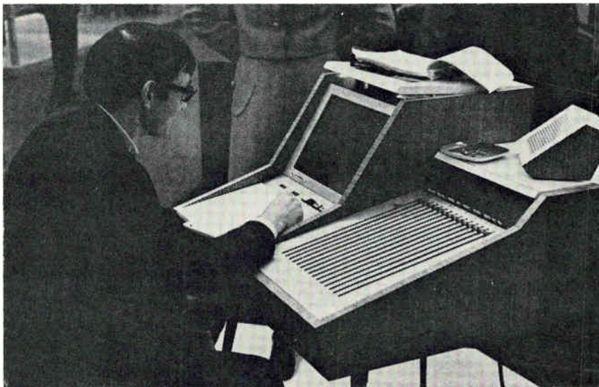
Am I right? Prospective customer ponders the merits of Sintra's machine, which, given a wrong answer, decides how many teaching steps to repeat.
