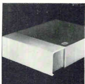
Parallel-input simplex modem 402C accepts 5, 6, or 8-level tape reader inputs and converts the data to parallel tones for transmission over the public telephone network. The modem is used in data collection systems and can be adapted to most parallel information applications. It operates at a speed of 75 characters/sec. General Data Comm Industries, Norwalk, Conn. [366]
