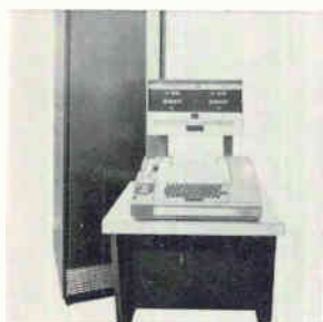
Algomatic 16 is a direct digital control and data handling system providing closed-loop control and data logging for 16 loops, expandable in 16-channel increments up to 128. Through its software, it processes the loop data using a control algorithm tailored to each loop. Data logging may be either full time or only for off-limit values. Research Inc., Box 24064, Minneapolis [361]
