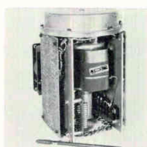
Disk memory system series 8100 has been developed to fit the mini-computer market segment that requires a combination of a compact and lightweight package with a bit storage capability approaching 145 K bits of storage. Package is 9 x 9 x 10½ in. Access time is 8.5 msec utilizing TTL interfacing. Information Data Systems Inc., E. Eight Mile Rd., Detroit, Mich. [363]
