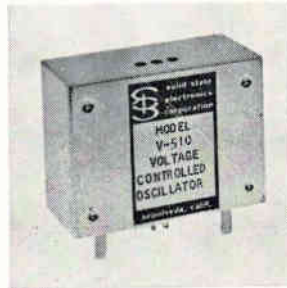
Voltage controlled oscillator V-510 is for accurate conversion or varying analog d-c voltage to a linearly proportional sine wave frequency. Standard units are calibrated for operation over a range from 400 hz to 70 khz within IRIG bands 1 to 18 ( \pm 7.5\% frequency deviation) and A to E ( \pm 15\% deviation). Solid State Electronics Co., Rayen St., Sepulveda, Calif. [343]
