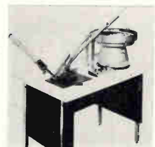
Dual in-line package insertion machine SM-2000 accepts DIP's from "sticks", loads them into carriers, and stacks the loaded carriers into magazines for further automated processing. It runs at rates up to 3,600 pieces per hour. Except for manual loading of carriers and DIP circuits, it is fully automatic. Weltek Div., Wells Electronics Inc., S. Main St., South Bend, Ind. [424]
