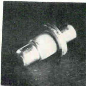
High power p-i-n diodes feature high dynamic Q switching in less than 300 nsec, high power handling capability, oxide and hard glass passivation, low C_T and high storage and operating temperature range. Units are recommended for use in r-f switching, limiting, phase shifting, duplexing and attenuating through Ku band. Microwave Associates Inc., Burlington, Mass. [441]
