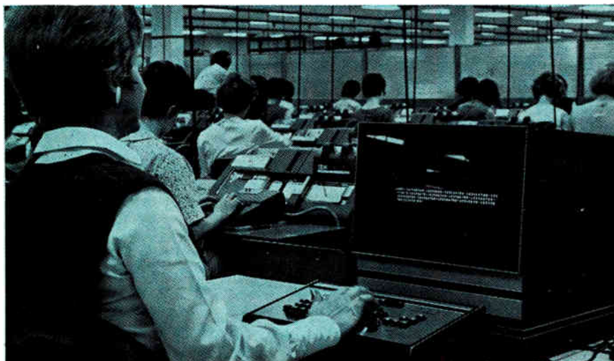
New media. Punched cards produced by the keypunches in the background are gradually yielding to other media, such as this General Electric Datatnet-760 terminal (shown in an Internal Revenue Service installation) for entering income tax data into a computer.
