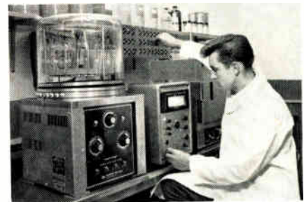
Volume and surface resistivity testing of copper-clad laminates. Exterior control unit, designed by Norplex, gives fast, reliable readout.
