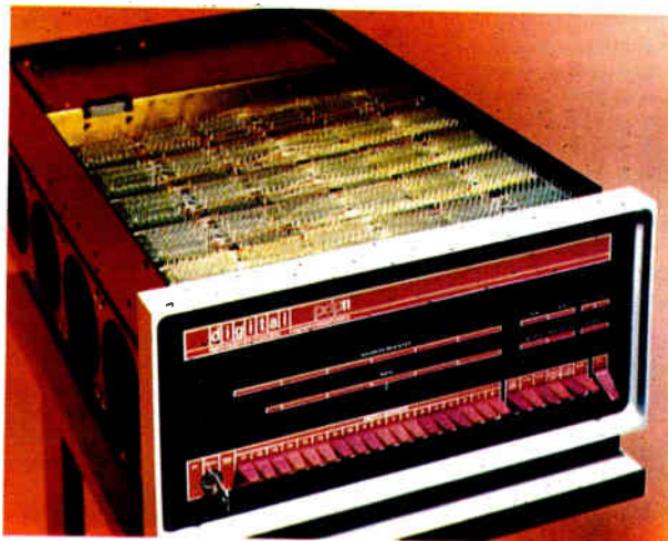
Expandable. The PDP-11, shown with top removed is modular in both physical and electronic design. Major subsystems such as the core memory, below, are easily removed and replaced.
