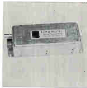
Logarithmic video amplifiers series LVA have a dynamic range in excess of 60 db for pulsewidths greater than 0.3 \mu sec and are available as unipolar or bipolar amplifiers. The design is based using feedback pair transistor amplifier stages whose feedback elements have exponential voltage-current characteristics. Locus Inc., 908 W. College Ave., State College, Pa. 16801. [383]
