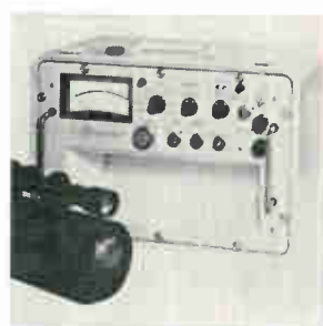
Precision radiometer 464 employs focusable reflective optics and reflex viewing for maximum convenience in field. It can be operated from a separate rechargeable battery pack (supplied) or power line or battery sources. Focus range is 10 ft to infinity; field of view, 1.5 milliradians; accuracy, \pm 2\% . Electro Optical Industries Inc., Box 3770, Santa Barbara, Calif. [363]
