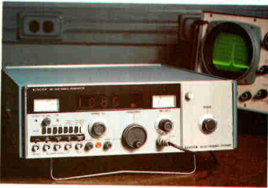
Inside or outside. The generator's built-in counter shows either the output's frequency or the frequency of some external signal.
