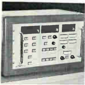
Disk test system designated Diskos I is for testing plated magnetic memory disks and drums. It displays all test parameters eliminating the need for oscilloscope viewing and operator calculations. Automatic head positioning and 3 test modes are offered: dropout, bulk properties and saturation. Diskos Electronics Corp., 201 Lonetree Ct., Milpitas, Calif. 95035 [365]
