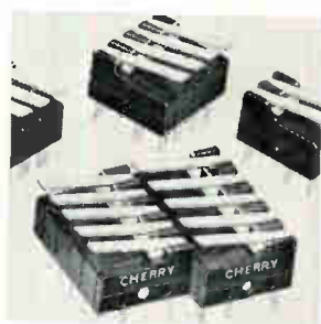
Subminiature switch modules provide multicircuit switching control, high electrical capacity and space economy. The series features 2, 3, 4 or 5-gang modules that are thinner than standard subminiatures. They are double-throw circuitry with ratings of 10.1 amps, 1/4 h-p, 125 v a-c. Cherry Electrical Products Corp., Old Deerfield Rd., Highland Park, Ill. [342]
