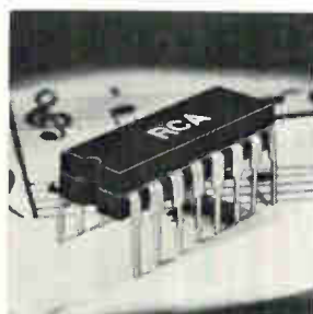
A-c amplifier array CA3052, on a single monolithic substrate, can be connected as a pre-amp to provide a high performance stereo tape head or full-function stereo amplifier. Each of four independent amps' typical operating features include an equivalent input noise voltage of 4\mu\text{v} and a high voltage gain of 58 db. RCA Electronic Components, Harrison, N.J. 07029 [442]
