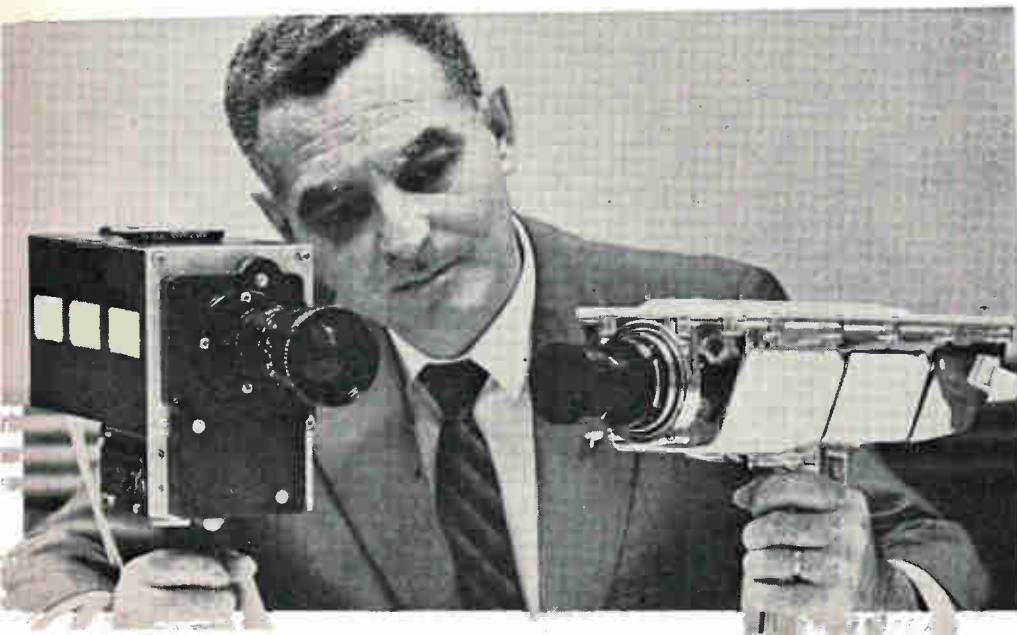
Space twins. Westinghouse's Apollo color camera, left, and the camera that took the pictures on the surface of the moon during the Apollo 11 mission use sec tubes developed for low-light-level tv applications.
