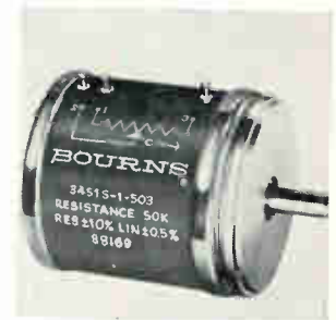
Servo mount precision potentiometer model 3451 is a 10-turn 2-in. diameter device featuring an Infinitron conductive plastic element. It has rugged element terminations, essentially infinite resolution, and a 50 million shaft revolution rotational life. Resistance range is 1,000 ohms to 500 kilohms. Power rating is 5 w at 70° C. Bourns Inc., 1200 Columbia Ave., Riverside, Calif. [344]
