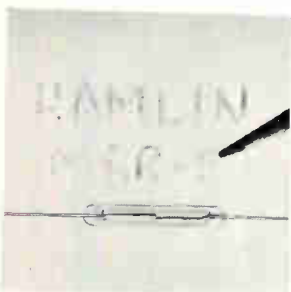
Magnetic reed switch MRR-5 is a single pole, normally open, Form A, and measures 0.130 in. max. glass diameter, 0.800 in. max. glass length, and 2.230 in. nominal over-all length, including leads. Initial contact resistance is 100 milliohms at 20 ampereturns overdrive. Maximum switching voltage is 500 v d-c; breakdown voltage, 1,000 v d-c. Hamlin Inc., Lake Mills, Wis. [345]
