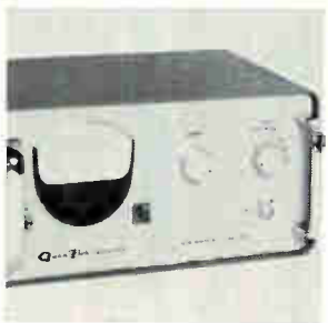
Random noise generator model 421 is designed to meet the need for an accurately calibrated noise source flat from 10 khz to 12.5 Mhz. To provide truly Gaussian amplitude distribution to better than 4 sigma and constant spectral density with frequency, the thermal noise of a resistor is used as the noise source. Quant-Tech Laboratories Inc., S. Jefferson Rd., Whippany, N.J. [366]
