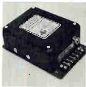
Power supply 3D5-2.5 for use with DTL, TTL and RTL logic uses 70% MIL parts. The calculated reliability per MIL-HDBK-217A is in excess of 150,000 hours. Input is 115 v a-c \pm 10\% , 60 to 400 hz. Output is 5 v at 2.5 amps; line and load regulation, \pm 0.3\% . Price (1-99) is $49 each. Powertec Div. of Airtronics Inc., 9168 DeSoto Ave., Chatsworth, Calif. [382]
