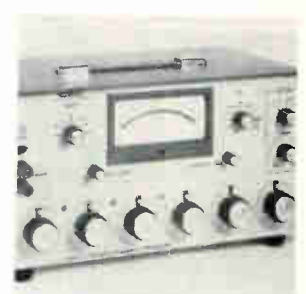
Wheatstone bridge WB-200B can also be used as a resistance comparator. It provides accuracy to \pm 0.005\% of reading and measurements of 0 to 110 megohms in 7 ranges. It combines in a compact and portable unit an all transistorized chopper, stabilized readout amplifier and an adjustable bridge voltage power supply. Precision Standards Corp., 1701 Reynolds, Santa Ana, Calif. [364]
