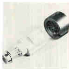
Series TS sockets are for test and burn-in applications of 8 and 10 lead TO-5 can IC's. Funnel entries guide leads into double-leaf, gold over nickel plated beryllium-copper contacts. One-piece bodies are molded from glass-filled diallyl phthalate good to 200° C. Contacts withstand many thousands of lead insertions and withdrawals. Robinson-Nugent Inc., New Albany, Ind. [347]
