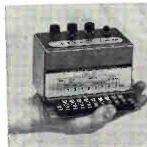
In less space than a desk phone occupies, a sold state extrasensory perception system can be installed to completely automate control of product flow in any production operation. The RM variable rate control module and a sensor work together to detect product flow and send signals to the scr motor controlling production line speed. PECO Corp., Ortega Ave., Mtn. View, Calif. [427]
