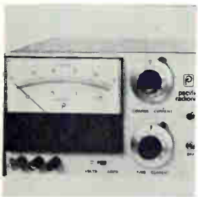
Constant current power supply model PP-21-6 was designed for YIG tuning applications. It provides up to 1 amp output current with compliance voltage up to 12 volts. Current adjustment is by two 10-turn digital dial controls providing 10 \mu a resolution. Unit features ripple and noise below 0.05 ma rms. Price is $225. Pacific Radionics Inc. 581 Division St., Campbell, Calif. [385]
