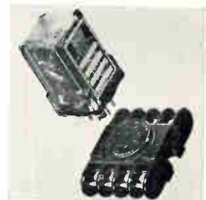
Plug-in dpdt control relay series ERB is comprised of an integral power supply, amplifier, transformer, output relay and circuit board, all in a case 2 1/2 x 1 3/8 x 1 3/8 in. It plugs into a standard 11-pin socket. The control instantly detects resistance changes in its input circuit from short circuit to 50 million ohms. Frost Electronics Corp., 1 Goddard Dr., Rockaway, N.J. [348]
