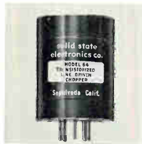
Plug-in line driven chopper model 64 incorporates a transformer-coupled isolating drive network and clipping diodes so that it can, for example, be driven from a 400 hz sine wave power line or from a drive source that is common to the d-c voltage being chopped. Unit utilizes a standard 7-pin header. Solid State Electronics Corp., 15321 Rayen St., Sepulveda, Calif. 91343 [343]
