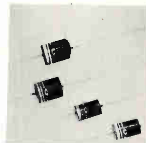
Wide area Varactron silicon voltage-variable capacitance diodes series VA521-824 feature all-epitaxial construction, Q as high as 200, and d-c ratings as high as 100 v. The devices are suited for such applications as vhf-uhf frequency multiplication, harmonic generation, oscillator tuning, and parametric amplification. Crystalonics Inc., 147 Sherman St., Cambridge, Mass. [439]
