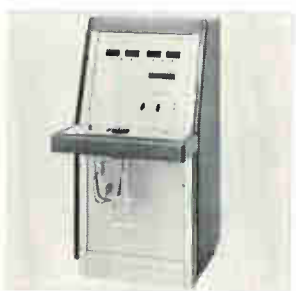
Automatic coil turns analyzer model 2000 check both turns and resistance. Accuracy for counting from 1 through 99,999 turns in an air core is guaranteed at better than 1 turn in 1,000 or \pm 0.1\% , whichever is greater. Resistance checks form 0.5 to 9,999.9 ohms are accurate to 0.5 ohm or 0.5%, whichever is greater. New Product Engineering Inc., Wabash, Ind. [367]
