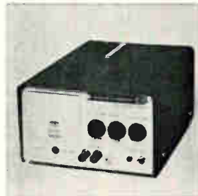
Parametric d-c power supply PDC incorporates the Paraformer which operates as a preregulator providing 1/4% regulation to the basic d-c unit, as well as more than 60 db filtering. Units offer \pm 0.001 v line regulation, 25 \mu sec response time, 250 \mu v ripple, and complete transient suppression. Prices start at $375. Wanlass Instruments, 1540 E. Edinger Ave., Santa Ana, Calif. [383]
