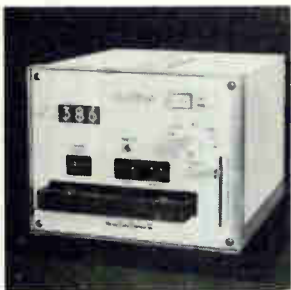
Digital recorder model DL620A contains a front panel presettable real-time clock; an 18-channel analog multiplexer; an analog to digital converter; a cartridge magnetic tape system with associated tape drive unit; plus all necessary logic and power supplies. System accuracy is 0.05% over 0° to 40° C. Metrodata Systems Inc., Box 1307, Norman, Okla. [421]
