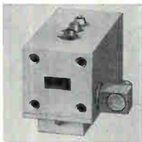
Millimeter diode switches series 750 are designed to operate in the 26.5-40 Ghz band. Spst and spdt types are available. Center frequency for the spst switch is 33 Ghz; bandwidth, \pm 3\% ; insertion loss, equal to or less than 1 db; isolation, equal to or greater than 30 db; switching speed, 10 nsec; price, $800. Control Data Corp., 400 Border St., East Boston, Mass. 02128 [402]
