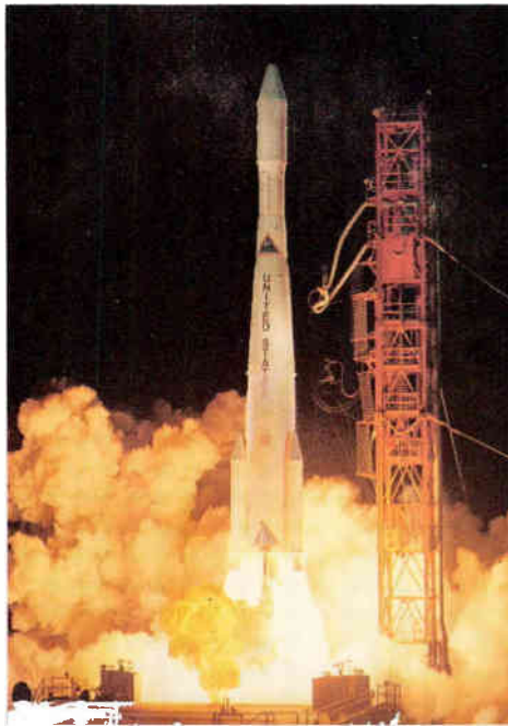
Excelsior. Tiros operational satellite heads for near-polar, sun synchronous orbit; craft surveys global weather conditions once every 24 hours, returning data and pictures to ESSA stations in Alaska and Virginia.
