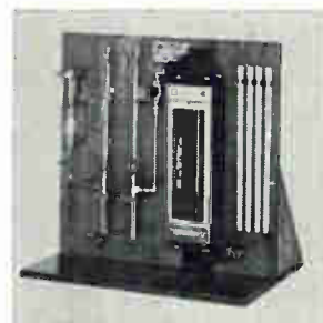
R-f calorimeter 6070 measures power in 50-ohm coaxial systems up to 5,000 w with 3% typical accuracy. Units are available with 1 1/2 in. EIA flanged connectors. Power is quickly and precisely determined from input-to-output temperature differential at a constant flow rate. Vswr is 1.1 max. (d-c to 1 Ghz); 1.2 to 2 Ghz. Bird Electronic Corp., 30303 Aurora Rd., Cleveland [407]
