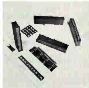
Digital strip indicators series 68020 are lighted readouts that display "0" through "9" in single or multiple decades. Units snap into panel cutouts and provide a built-in appearance. Light sources are T-1 3/4 flange based lamps, incandescent or neon (10 lamps per decade), which are front panel replaceable. Cartelli Technology Inc., 41-10 102nd St., Corona, N.Y. 11368 [347]
