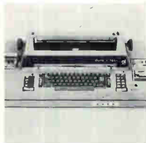
Data terminal 1051 bridges the gap between portable terminals with dial-up capabilities only and permanently located desk-structured, multiunit terminals providing automatic data transmission as well. The unit is compatible with 360 systems and can replace 360 data terminals or operate with them without software charge. Intercontinental Systems Inc., Palo Alto, Calif. [426]
