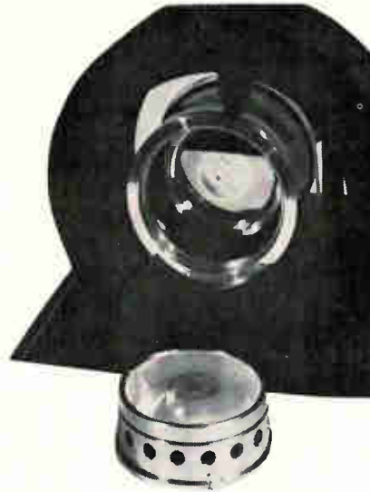
The means. This is a feasibility model of the electron tube to be used with electron-beam masking machine developed by Westinghouse to be built and sold by Hugle.
