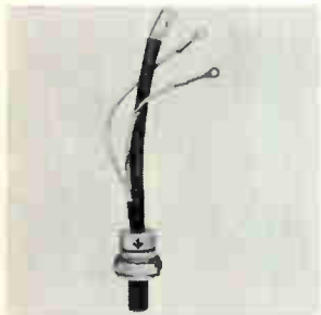
Silicon controlled rectifiers 2615 and 2605 will operate at a junction temperature of 150° C. The 2615 has a forward current of 200 amps rms and is rated at 125 amps half-wave average. The 2605 has a forward current of 275 amps rms and is rated at 175 amps half-wave average. Both have guaranteed dv/dt of 300 v per μsec. Westinghouse Electric Corp., Box 868, Pittsburgh [440]
