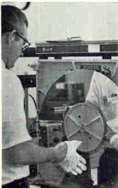
Test. Videotape transport is checked by technician on Ampex assembly line.
