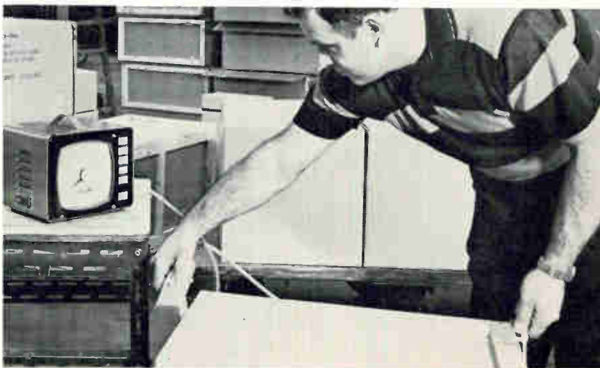
Automated tape measure. Uncoiling steel wire in hand-held probe turns potentiometer which delivers a voltage proportional to dimension.
