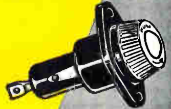
HPC-C panel mounted holder, visual-indicating, for \frac{13}{32} x 1\frac{1}{2} in. fuses.
