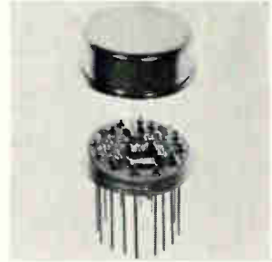
Precision ladder switch has a typical switching speed of 380 nsec. Miniaturized to fit two switches into a sealed TO-8 can, the hybrid circuits come in 8 basic types to meet a variety of requirements. Offset voltages are prebalanced to two ladder current ranges: 1.6 ma to 3.5 ma or zero to 1.6 ma. Maximum offset is \pm 2 to \pm 4 mv. Mepco Inc., Morristown, N.J. [348]
