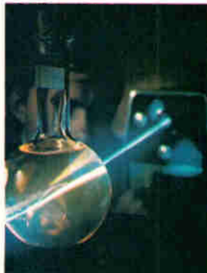
New blue. Beam from helium-cadmium laser strikes an organic solution in a flask, causing fluorescence. The metal-vapor system is expected to be used initially in biochemistry and photochemistry.
