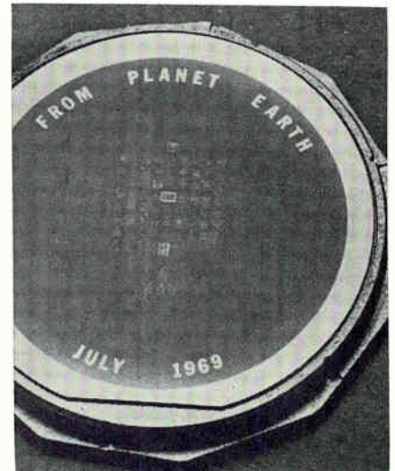
Compact. This is message disk for Apollo 11. It carries 87 messages at 1/200th size on a 1.5-inch disk of pure silicon.
