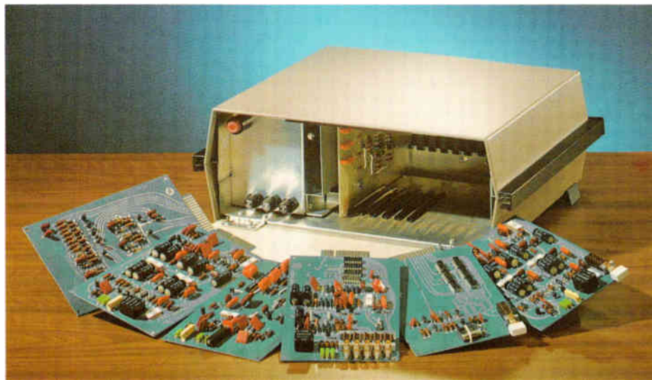
Best seller. Since the Carterphone decision, the hottest thing in the communications field has been modems. Among the units on the market is Ultronic's Series 2400 Data Pump, which receives and transmits synchronous digital data over voice-grade phone lines.
