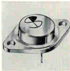
Silicon high-power transistors with collector-emitter voltages up to 300 v come in the JEDEC TO-3 package. They feature power dissipation at 25° C of 350 w, extremely low saturation resistance (as low as 0.30 ohm) as well as low leakage currents and thermal impedance. Maximum collector current is up to 30 amps. Solid Power Corp., 440 Eastern Pkwy., Farmingdale, N.Y. 11735 [438]
