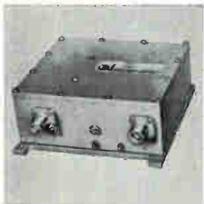
Solid state, crystal controlled pulsed r-f source model S-1001 is a 150-watt unit that covers a frequency range of 100 to 500 Mhz. Frequency stability is rated at \pm 0.005\% and duty factor at 10% maximum. Unit operates from a +28 v d-c power supply and in a nominal temperature range from -40^\circ to +71^\circ C. Aerodyne Industries Inc., Willow Grove, Pa. 19090 [401]
