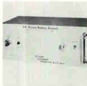
True digitally programmable millivolt calibrator model MV-100P is programmed from BCD logic signals. Various programmers may be used, such as: punch tape, punch card, incremental magnetic tape readers, or key board. Full scale output voltage is 166.65 mv. Resolution is 10 \mu v. Accuracy is \pm 0.015% of setting \pm 5 \mu v. Electronic Development Corp., 423 W. Broadway, Boston 02127 [422]
