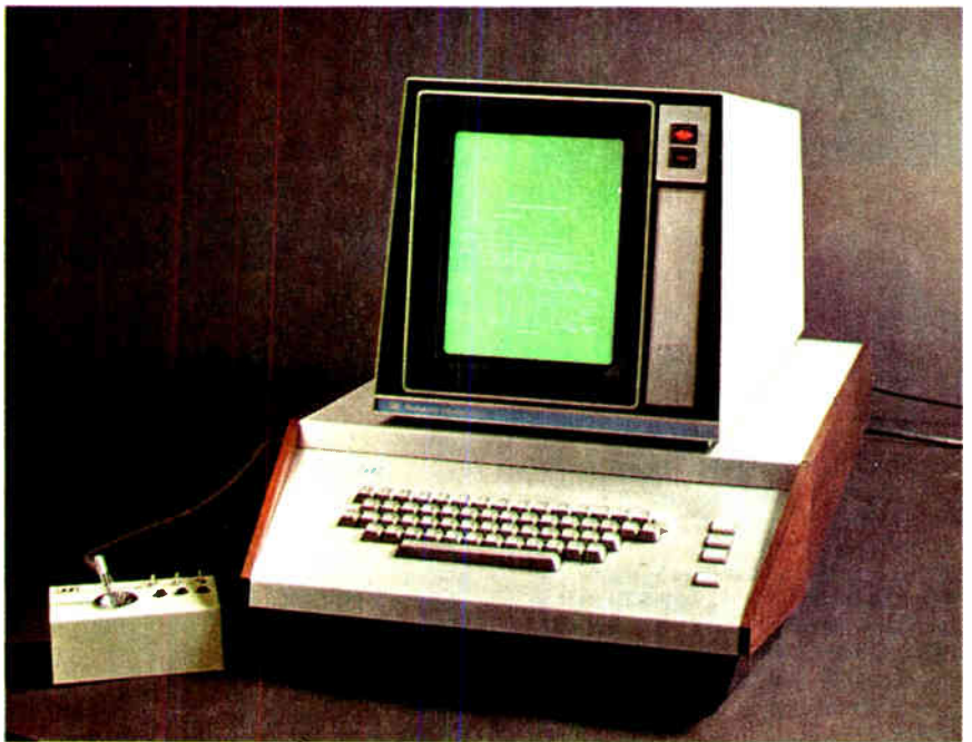
Versatile. Terminal can display schematics as well as alphanumerics. Joystick at left is used as position controller in design work.
