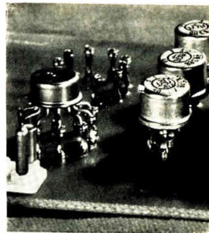
Adaptable. Individual terminals produce custom-made transistor sockets.
