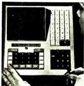
Compact crt computer terminal model 2212 is for processing short messages between non-typist operators and computers. It has an integral 6-in. crt for data display, block alpha and block numeric key clusters, and a cluster of 24 editing and programable function keys. Screen can display up to 444 characters on 12 lines. Bunker-Ramo Corp., 445 Fairfield Ave., Stamford, Conn. [361]
