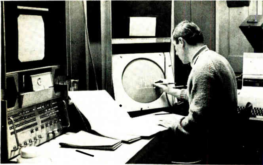
Light writing. Heinz Lemke of the Cambridge University Mathematical Laboratory developed the command scheme for the Pixie CAD system. Only the light pen—there are no buttons to push—is used to change designs.
