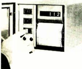
Compact digital logging instrument model DL-1210 Digilogger is designed to accept virtually any analog signal from 1 to 30 check points and provide numerical print-out. Basic unit consists of a 50-channel scanner, an automatic 12-column paper roll and ink printer, plus the necessary solid state electronics for conversion. Entex Inc., P.O. Box 770, Friendswood, Texas 77546. [365]
