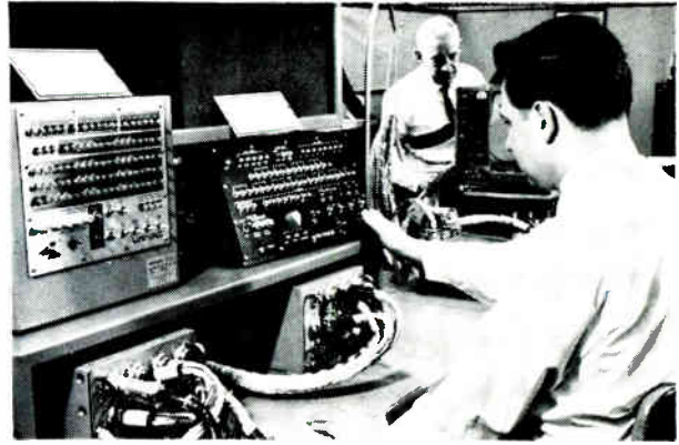
Bench test. Sperry engineers decided early in the Navy ILAAS program to integrate four major electronic subsystems through a central computer complex. Here the inertial-radar-data computer control panel (left) and flight-test memory panel (upper shelf) are tested, while the staff member in the background checks out the system's inertial reference set.
