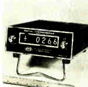
Multiple channel digital thermometer model 903 offers direct read-out and covers the range of -60^\circ to +160^\circ C. It has a guaranteed accuracy of 0.5^\circ C, and a resolution of 0.1^\circ C with memory display. Ten input channels are controlled by a master channel selector switch. Unit measures 2\frac{5}{8} \times 6\frac{3}{4} \times 9\frac{1}{2} in. Electronic Research Co., W. 75th St., Overland Park, Kan. [386]
