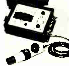
Infrared radiation pyrometer/controller called Industrial Pacemaker permits sensing the temperature of a workpiece or material in process of fabrication, without touching it. It covers the temperature range 1000^\circ to over 4000^\circ F with several convenient models. Unit is housed in a vapor tight cabinet for severe environments. Irtronics Inc., 57 Commerce Road, Stamford, Conn. [387]
