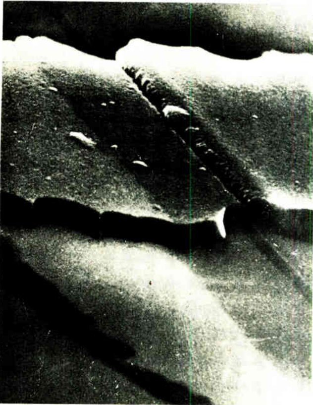
Fissured floes? No it's an aluminum interconnect strip cracked where it passes over an oxide step on a Fairchild IC. At right is one that isn't cracked. The photo at left is a 10,000 X magnification, the other is 20,000 X.
