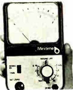
Miniature meter model TM1 measures the time interval between opening and/or closing of contacts. Time range is 1 msec to 10 sec in 9 ranges. The readings are maintained for at least 1 minute on the 3-in. linear scale. Accuracy is \pm 2\% full scale deflection. Unit weighs 1 lb 4 oz, measures 5\frac{3}{4} \times 3\frac{3}{4} \times 1\frac{3}{4} in. Amstro Corp., 120 Clinton Rd., Fairfield, N.J. [382]
