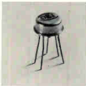
Monolithic timing circuit model 7100 is for any type of timing application, from monostable delay circuits to turn-on delays. Features include: 10 \mu sec to 1 hour time delays; only 1 to 2 external components required for the majority of applications; and output compatible with 10 volt analog, MOS, RTL, DTL and TTL forms of logic. Optical Electronics Inc., Box 11140, Tucson. [441]
