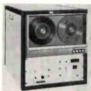
Data acquisition system model 710 can multiplex and digitize 64 channels of low-level analog data onto magnetic tape. It contains a 16-channel FET multiplexer which is expandable to 64 channels with a switching speed of 1 \mu sec/channel. Accuracy of the integrating digitizer is 0.015% of full scale at 15 msec/conversion. IRA Systems Inc., 332 2nd Ave., Waltham, Mass. [423]
