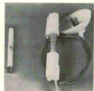
Selenium high-voltage rectifier TV18-TOK70 for black-and-white tv application features high life expectancy. The 24 kv piv rectifier has the length of a comparable h-v tube rectifier, 2 3/4 in. The baseplate material has a thickness of approximately 0.003 in. compared with 0.012 in. of standard material used until now. ITT Semiconductors, 6416 W. Belmont Ave., Chicago 60634. [443]
