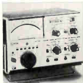
Model PM6509 meter performs leakage current, breakdown voltage and resistance measurement in pico and nanoamp regions without auxiliary equipment. Current measurements down to 3 pa, breakdown voltage up to 1,000 v and resistance measurements up to 100 teraohms are accurately performed. Price is $1,100. Philips Electronic Instruments, Mount Vernon, N. Y. [366]
