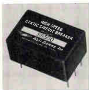
High-speed, d-c static circuit breaker, model SD500 gives a clean, arc-free, bounceless break at 50 \mu sec after current overload. It is available in 5 models, ranging from 25 ma to 1 amp. Each has its trip point adjustable from 50% to 150% of its rating. Price (1 to 3) is $26.75 each; delivery, stock to 2 weeks ARO. Flight Systems Inc., P.O. Box 25, Mechanicsburg, Pa. 17055 [341]
