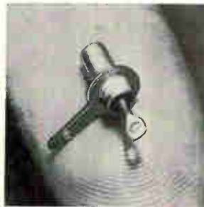
Gas-filled metal diodes serve as protective devices against transients or other sharp spikes, such as those which can puncture MOS FET's. Inherent firing voltage is 80 to 89 v. Leakage resistance is greater than 3.5 \times 10^{14} ohms. Repeatability of firing voltage is approximately \pm 5\% and self capacitance 1.1 pf at 100 khz. Victoreen Instrument, 10101 Woodland Ave., Cleveland. [438]
