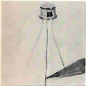
Triple-diffused silicon power transistors series SDT4921-SDT4925 are 300-v, 5-amp devices in TO-5 cases. They feature ultrasonically bonded leads and gold silicon eutectic die mounting. Beta at a collector current of 1 amp is a minimum of 20 and a maximum of 60. Collector to emitter voltage is less than 0.5 v. Solitron Devices Inc., 1177 Blue Heron Blvd., Riviera Beach, Fla. [440]
