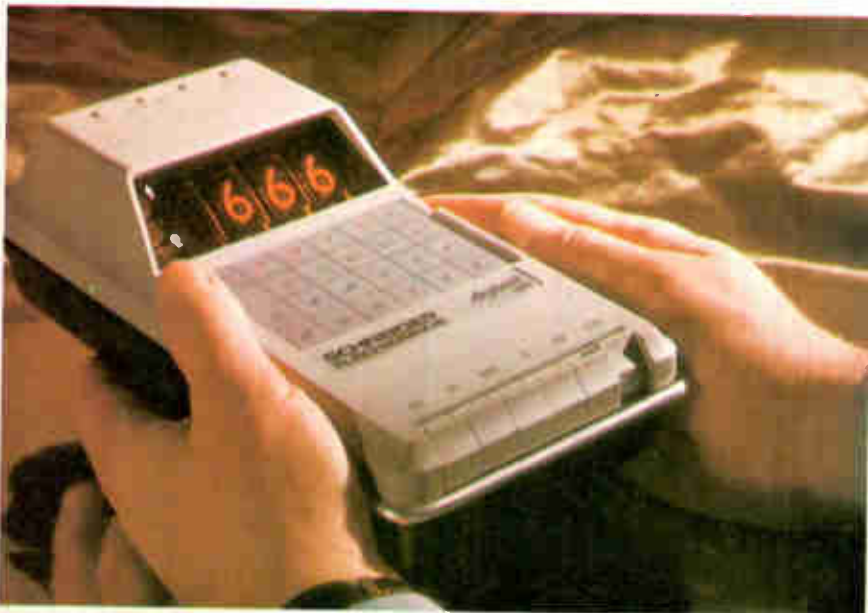
Frank display. The price of this three-digit multimeter is $195. Schneider, the meter's maker, kept costs down by using a custom-designed LSI circuit in place of a dozen off-the-shelf IC's. The meter has 17 ranges, and runs off line voltage or a battery.
