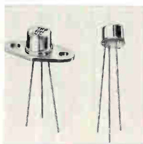
Complementary npn and pnp transistors in both TO-5 and MD-14 packages are available at up to 800 v. Average beta of the NPN's is 15,000 at a collector-to-emitter voltage of 10 v and collector current of 20 ma. Average beta of the pnp's is 20,000 at a collector-to-emitter voltage of 10 v and collector current of 10 ma. Industro Transistor Corp., 35-10 36th Ave., L.I.C., N.Y. [438]
