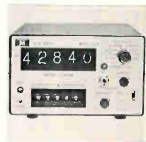
Operating modes of the model 104A counter include: direct totalization from 1 to 10^5 ; preset totalization, with all 5 decades presettable from 0 to 9; "rate", in which gate times are selectable from 1 \mu\text{sec} to 100 sec for normalized readings. Basic counting range is from 5 hz to 8 Mhz. Price is $850. Monsanto Co., 620 Passaic Ave., West Caldwell, N.J. 07006. [364]
