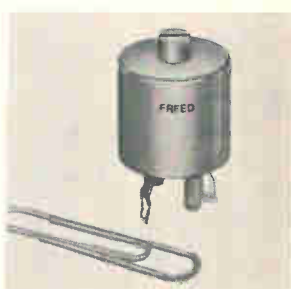
Variable high-frequency inductors feature a Q of 500. Types VHI-1 through VHI-10 have an inductance range of 1 mh to 50 mh, and a frequency range of 50 khz to 500 khz. Types VHI-11 through VHI-22 have an inductance range of 9 \mu\text{h} to 600 \mu\text{h} and a frequency range of 100 khz to 10 Mhz. Freed Transformer Co., 1718 Weirfield St., Brooklyn, N.Y. 11227. [348]
