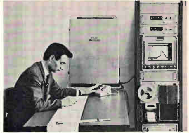
In depth. Depth-distance logged by survey ship gets converted into river-bottom profile by shore-based computer. System does the job in days; hand plotting takes weeks or months.
