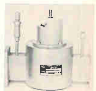
Tunable transmission reference cavity 40A141700 covers 5.925 to 6.425 Ghz with a stability of ±250 khz over a temperature range of -15°C to +65°C and stability of ±0.0005%. Insertion loss is 2.0 db max. Nonoperating environmental conditions include 20G shock and 10 to 55 hz vibration at 10 G acceleration. Frequency Engineering Laboratories, Box 527, Farmingdale, N.J. [404]
