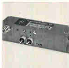
Solid state voltage controlled oscillators series FS-18 are available in C and X band with two options. The standard FS-18 will cover any selected 500 Mhz band within 4.8 to 11 Ghz with power output of 5 to 25 mw. The FS-18 W has an 1,100 Mhz bandwidth capability within 8.5 to 11 Ghz with power output of 1 to 5 mw. Frequency Sources Inc., N. Chelmsford, Mass. [402]
