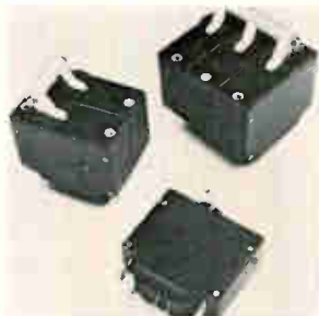
Magnetic circuit breakers series 51MC come in ratings from 0.020 to 50 amps, a-c or d-c, in single and multipole versions. Multipole types have an internal tripping action so that a fault in any pole will trip all poles. Units are available in relay and shunt-type configurations as well as the standard series type. Texas Instruments Inc., 34 Forest St., Attleboro, Mass. [342]
