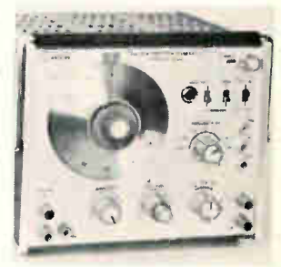
Solid state function generator PM5168 offers 3 simultaneous fixed amplitude waveform outputs (square-, triangle- and sine wave) over 7 frequency ranges, from 0.0005 hz to 5 khz. A fourth output can be switched to provide any of the 3 waveforms with adjustable amplitude and d-c reference level. Philips Electronic Instruments, 750 S. Fulton Ave., Mount Vernon, N.Y. [368]
