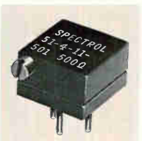
Plastic case \frac{3}{8} -inch square trimmer model 51 meets MIL-R-27208. It is available with resistances in the 10 to 50,000 ohm range. Features include light weight (1.5 grams, max.), a 200-cycle rotational life, resistance tolerance of \pm 5\% , and a power rating of \frac{3}{4} w at 85 ^{\circ}\text{C} . Price in 1-9 quantities is $4.81. Spectrol Electronics Corp., E. Gale Ave., City of Industry, Calif. [346]
