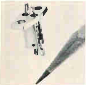
Magnetically actuated spst switch is for positive operation as low as -423^{\circ}\text{F} and under vibration conditions of 45 G. It senses any linear or rotary valve, shaft or rotor position. Shock to 100 G will not result in a discontinuity greater than 10 \mu\text{sec} . The contact is rated at 2 amps inductive at 28 v d-c. Kinetics, a Teledyne Co., 410 S. Cedros Ave., Solana Beach, Calif. 92075. [341]
