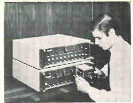
Noisemaker. Test set measures distortion in voice network.
