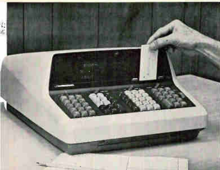
Program card. An operator loads a magnetic card containing a previously written program into the calculator's card reader.
