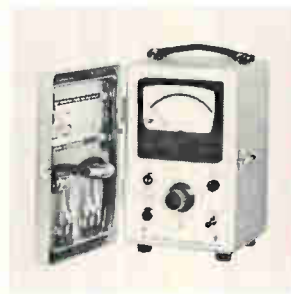
Portable milliohmimeter model 502A offers 30 \mu\text{ohms} sensitivity and less than 2 \mu\text{w} power dissipation. Accuracy is 3% of full scale. Full scale ranges are from 0.001 to 1,000 ohms. Maximum voltage across sample is 25 mv peak-to-peak. The unit is battery operated with a minimum of 360 hours battery life. Price is $495. Keithley Instruments Inc., 28775 Aurora Road, Cleveland. [363]
