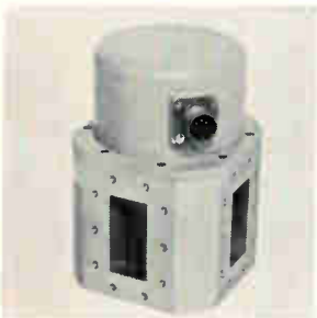
Waveguide switches series 77 are driven by a 28 v d-c solenoid actuator and held in place by a holding circuit. They cover the frequency range of 2.6 to 40 Ghz. Units are available in four port, E or H plane versions, with both interlock circuiting and fail-safe return mechanism. Prices range from $365 to $995. Waveline Inc., P.O. Box 718, West Caldwell, N.J. [401]
