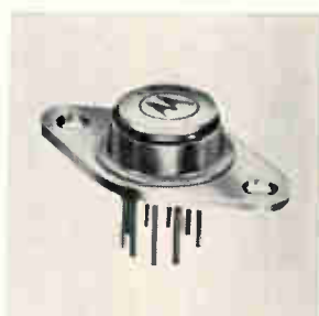
Monolithic voltage regulator type MC1560 is designed to deliver load current up to 500 ma without use of an external power transistor. It has 0.002%/v typical regulation with changes in input voltage, and 20 milliohms output impedance for excellent load regulation. Power dissipation is 10 w max. at 65°C. Motorola Semiconductor Products Inc., Box 955, Phoenix 85001. [443]
