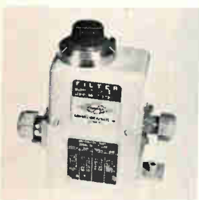
Six-section gang-tuned filter model G642 has a maximal flat response and is tunable from 3.7 to 4.2 Ghz. Rejection is 40 db minimum at a resonant frequency of ±70 Mhz, 60 db minimum at a resonant frequency of ±120 Mhz. Insertion loss is 0.6 db max. Maximum vswr over a resonant frequency of ±18 Mhz is 1.4:1. Gombos Microwave Inc., Webro Road, Clifton, N.J. [405]
