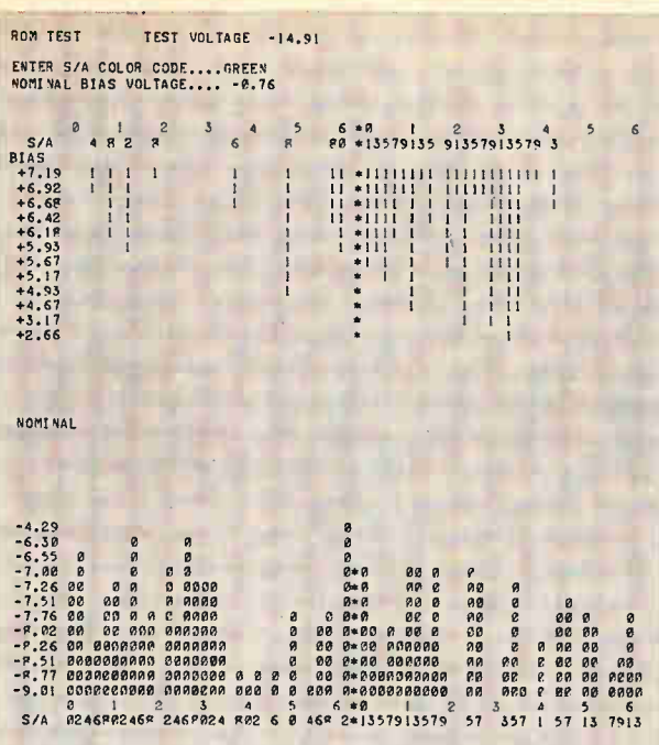
Margin profile. Failing sense amplifiers are listed over a range of sense-amplifier bias voltages. The open space in the middle indicates the width of the operating "window"—9.22 volts for the even-numbered amplifiers (left) and 9.66 volts for the odd-numbered ones.
