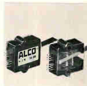
Double pole, subminiature reversing snap-switch model ML2-70 has two butterfly double-break mechanisms. Use of snap-action provides a quick make-and-break of controls in each circuit. Current rating is 3 amps at 125/250 v a-c; operating force, 75 to 100 grams; lever length, \frac{3}{8} in.; life cycle, 500,000. Alco Electronic Products Inc., P.O. Box 1348, Lawrence, Mass. 01843. [344]
