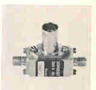
Coaxial switch model M405 covers 1 to 18 Ghz with over 40-db isolation above 8 Ghz, 0.5 to 2.5 db insertion loss, and 2 w c-w and 100 w peak power. Applications include: general-purpose 50-nsec laboratory switch, pulse modulator and shaper, amplitude modulator, limiter, automatic gain and level control. Somerset Radiation Laboratory Inc., 2060 N. 14th St., Arlington, Va. [408]
