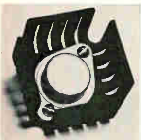
Heat sink model LP12 measures 1.60 x 1.60 x 0.75 inch with less than 1 mil surface smoothness. It will dissipate 16 w for 100 ^{\circ}\text{C} temperature rise. It can be ordered with no finish, conversion coating, gold iridite, black or hard anodized insulated for 500 v, and can be stamped for TO3 or TO66 transistor outline. TOR Inc., 16329 East Arrow Highway, Irwindale, Calif. 91706. [345]
