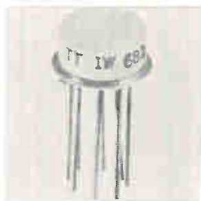
Audio amplifier IC in a TO-78 package is applicable to any product or system requiring low distortion audio output power from milliwatts to the one-watt level. It is operable from a 6 to 20 v d-c supply, temperature compensated from 0° to +85°C, and has an input impedance of 400 kilohms. Trans-Tek Manufacturing Co., 4405 S. Clinton Ave., South Plainfield, N.J. 07080. [437]
