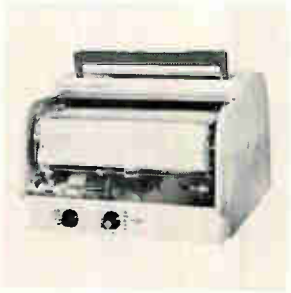
Portable potentiometric recorder's chart speeds can be changed with a finger-tip selection feature with electrical selection of inches per hour or inches per minute. This gives a choice of 10 different chart speeds. Maximum accuracy is assured with readings of 0.25% of full scale or \pm 5 \mu\text{v} , whichever is greater. West Instrument Corp., N. River Road, Schiller Park, Ill. 60176. [367]
