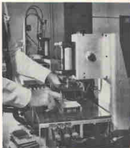
Reliability assured — through 100 percent electrical test of every board.
