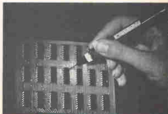
Visual aid. Presence of logic pulse is indicated by lighted band near tip.
