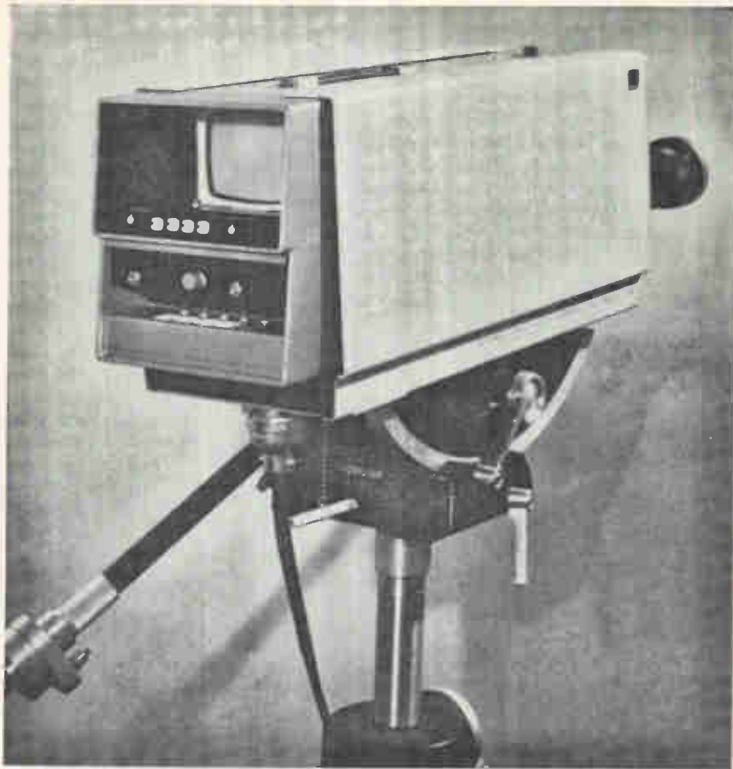
Self-contained. Equipped with three separate mesh vidicons, the camera includes 6:1 zoom lens, external color encoder, studio junction box, and remote controls.
