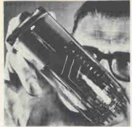
Sharp-eyed. Photomultiplier can detect a light-producing nuclear event that generates only a single electron.
