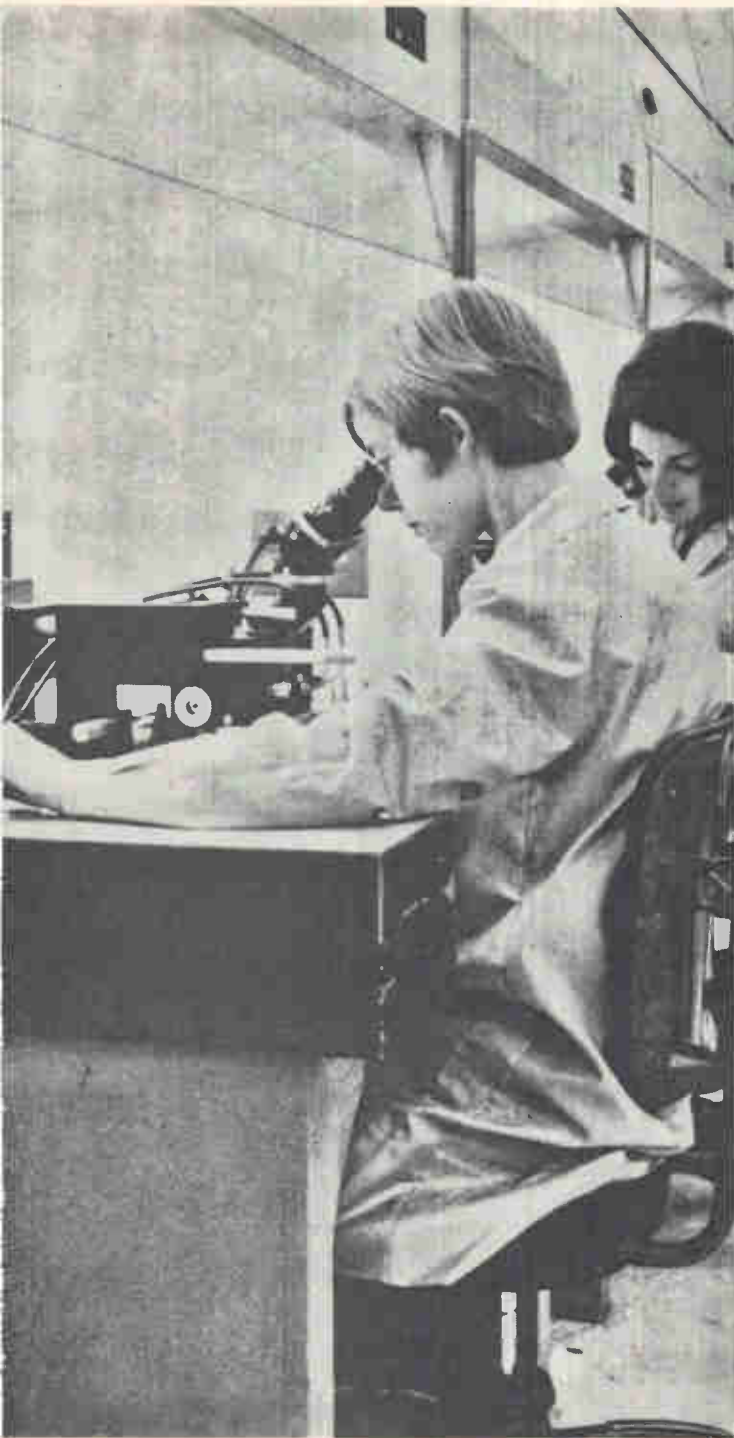
Key operation. Looking at the wafer through a microscope, the operator positions the photolithographic mask with a joy stick. Procedures like this require skill and elaborate precautions against contamination.
