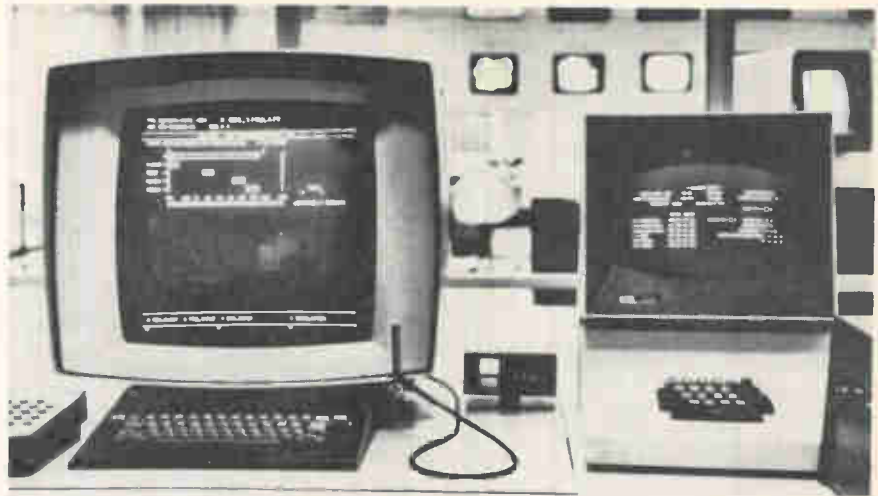
New way. Visual display units replace memo pads in NHK's information and control system. The IBM 2250 at left presents data in chart form, in this case dates and duration of rehearsals. The IBM 2260 at right displays information being displayed on another terminal elsewhere.
