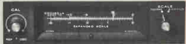
Switch-selected meter modes, normal or expanded scale, provide level measurement resolution of 0.05 dB. Signal generator level increments as fine as 0.01 dB can be readily resolved.
