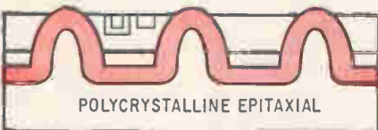
DIFFUSION OF BASE, EMITTER AND TOPSIDE COLLECTOR CONTACT BY THE NORMAL METHOD
