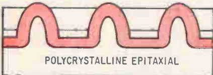
WAFER FLIPPED OVER AND N MATERIAL REMOVED BY MECHANICAL POLISHING, ETCHING OR BOTH
