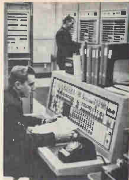
Check point. Status display console rides herd on communications and data processing portions of the Buic 3; system serves as maintenance monitor.
