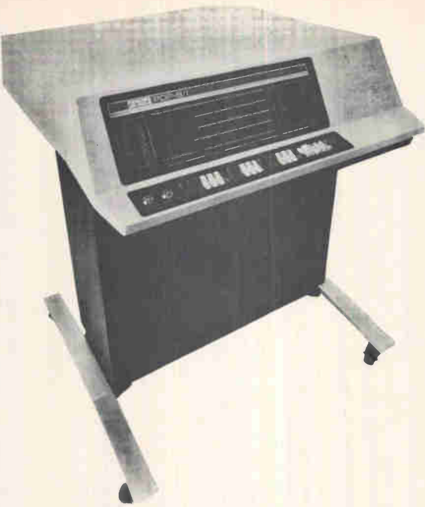
Little giant. This computer, the all-IC PDP-8/I, can be more powerful than the discrete version because it has room inside for several optional features. It's small enough for a desk top.
