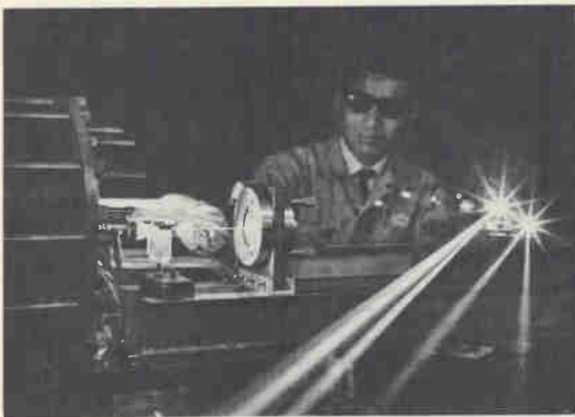
Turned on. A technician checks multicolored rays emitted by what Japan's Tokyo Shibaura Electric Co. says is the first long-life, high-output argon and krypton lasers made in Japan. They can oscillate over 11 wavelengths from blue to green; total output is one watt. Beryllium ceramics, rather than quartz, are used for the tubes.
