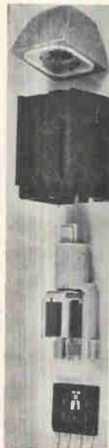
Button action. Lead frame with four terminals, at bottom, has IC mounted near top edge. Just above it is plunger with magnet which surrounds chip and actuates circuit. At top are key button and, under it, the switch housing.
