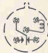
1 Form C, all contacts insulated from case
