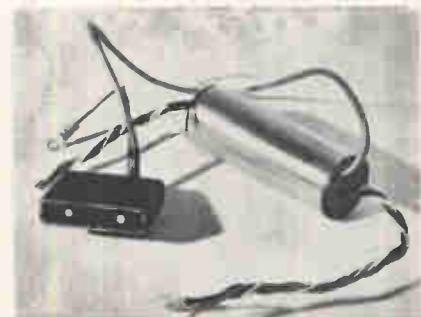
Sentry. A reed switch in the cylindrical package closes when a light fails, and the red panel light comes on.
