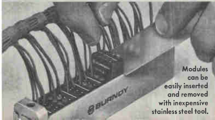
Track features recessed mounting hardware so there is no interference with removal of modules. Two-piece end clamp construction permits insertion from ends or top anywhere along track.
