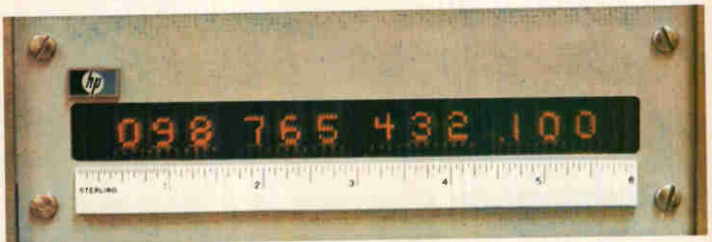
Sharp definition. With a red glass cover, the IC and the metalization are not visible, and the diode display appears to float in space.
