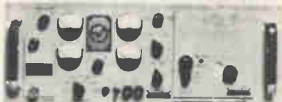
1037-G . . . 55-2300 MHz tuning range. Solid state with nuvistor and stripline tuners. Matched IF filter/demodulators. All IRIG bandwidths. Optional SDU and up/down converters.
