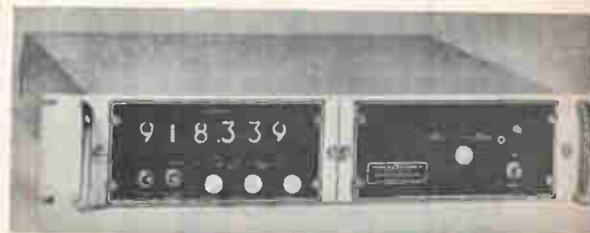
Stretchout. Extender, at right, pushes counter's range up another 700 Mhz.
