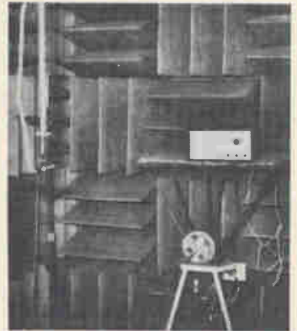
Sounds of silence. Radio receivers are checked out in an anechoic test chamber at electronics division's laboratory.
