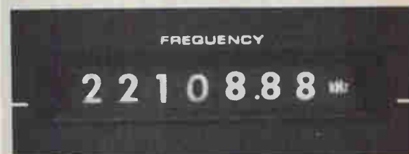
Frequency resolution to nearest 10 Hz in phase-locked tuning mode is displayed on flat-plane, high-brightness readouts. Alternative continuous tuning mode presents frequency resolved to nearest 100 kHz.
