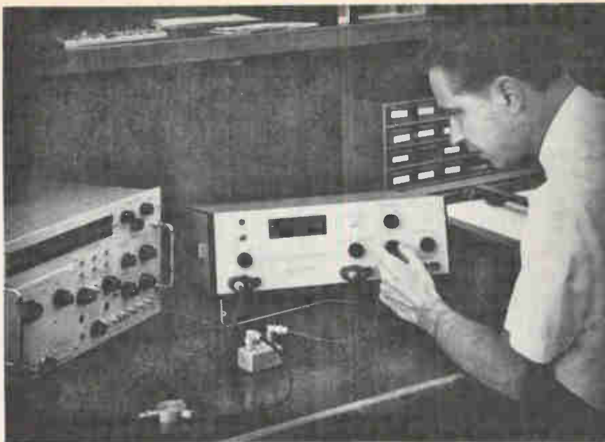
Wide-ranging. Phasemeter covers band from 10 hertz to 2 Mhz. Range makes it useful for measuring response of feedback circuits.
