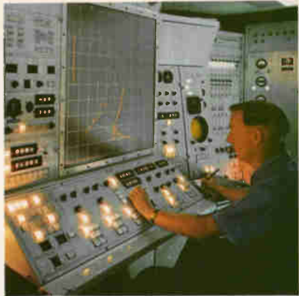
Warfare trainer. Display system helps train helicopter crews in antisubmarine warfare by plotting up to five separate sonar targets. It also displays simulated flights and actual ASW exercises. System is mounted in van.
