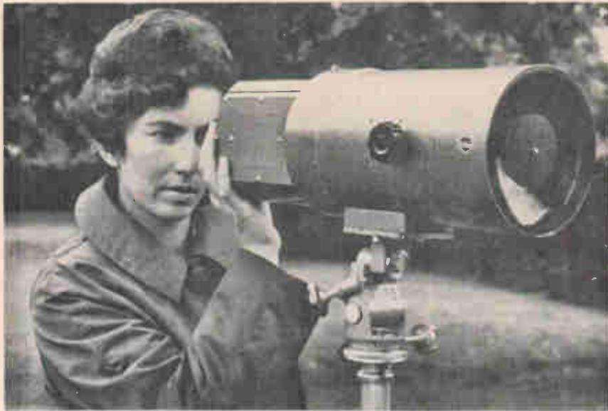
Good looking. Mullard's Daphne Lamport checks the scene with a demonstration night-viewer built around a recently declassified image intensifier tube. Early development of the tube was performed by a team headed by Miss Lamport.
