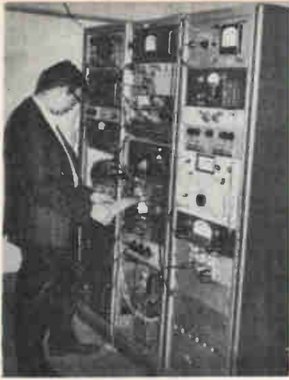
Checkup. Arnold Seligson, an audio specialist watches recorder unit plot bandpass curve of a receiver under test at Consumers Union lab.
