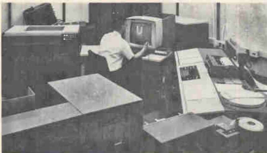
Custom design. Gleam is a low cost IBM system for computer-assisted design. It uses an IBM 1130 computer, a 2250 display unit, plotter drafting machine, and a precision controller.
