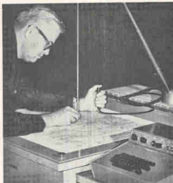
Tracing table. When graphic information isn't available on a slide the operator can trace the picture; the system automatically makes a slide.
