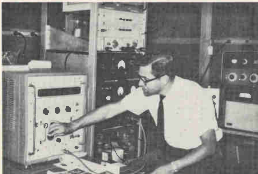
Switchover. To rate speakers, an operator shifts output among several while a record plays so the panel can determine which perform the best.
