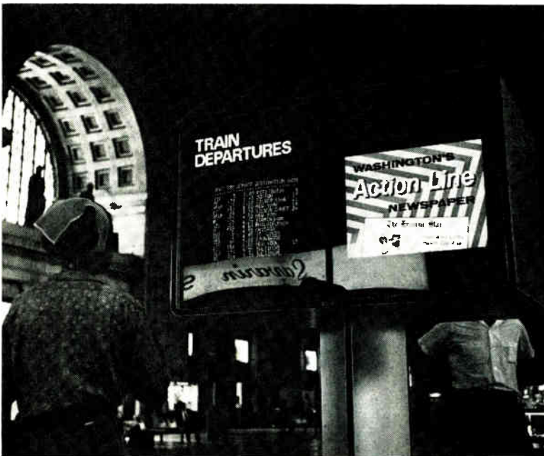
On display. The A.B. Dick Co. has long been known for its duplicating and copying machines. But now, as a result of spin-off from its electrostatic high-speed label-printing equipment, the firm has entered the electronic data-display field with this unit, the Videograph Series 900. It can present up to 512 characters in 16 rows directly from a keyboard or a computer. This installation is at Penn Central Station in Washington.
