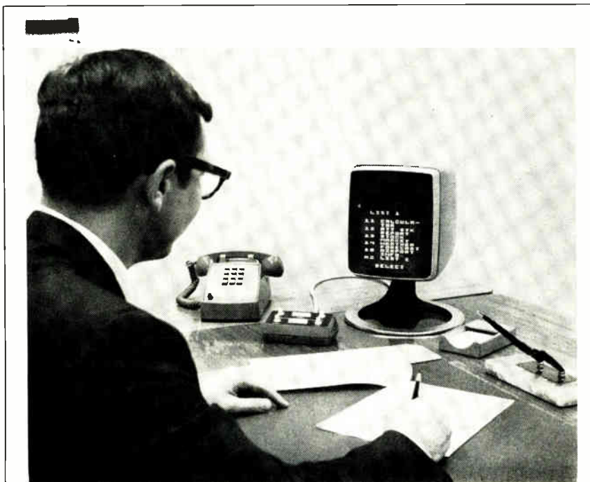
Ring up a computer. Engineers at Bell Telephone Laboratories in an in-house experiment, linked an unmodified commercial computer to this Picturephone so their device could be used as a desk terminal to display data on such things as inventories and news, stock, and weather. Bell plans additional tests; no marketing plans have been made.
