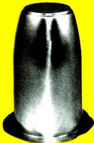
Brass 70-30; 12" diameter, .35" blank One draw • 12,000 psi
