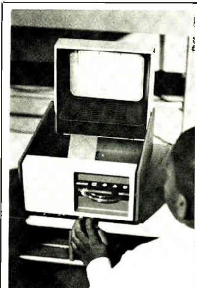
Teacher. CBS Laboratories and the Reading Institute of Washington, D.C., have developed this $350 programed learning system, the AVS-10. Video—152 transparencies—line the outer edge of record; record has 600 lines per inch, plays at 22½ rpm. Response is 100 to 7,500 hertz. Slots on the cartridge operate microswitches to provide answers to questions.
