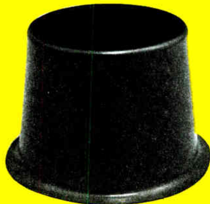
Stainless Steel 304; 12" diameter, .030" blank Two draws • 14,000 psi
