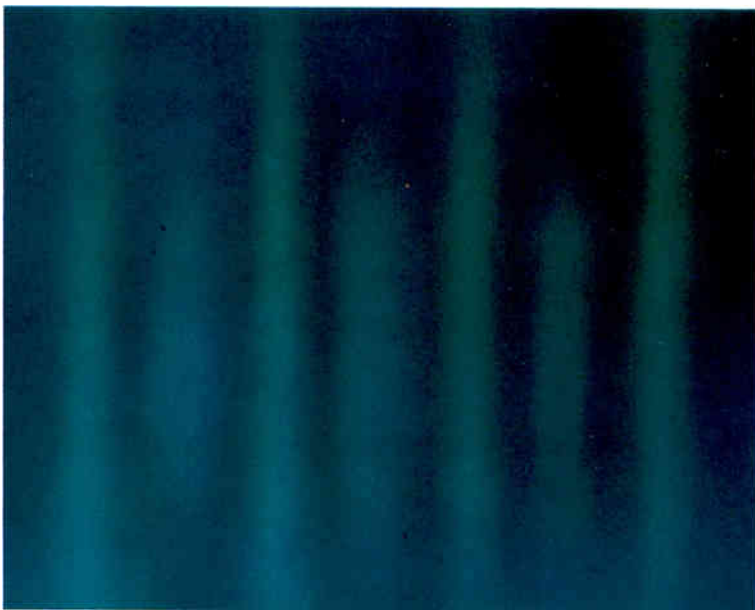
On the fringe. Young's fringe pattern was produced here by putting a film packet at the convergence point of beams from two X-band horns set at a 90° angle to each other.
