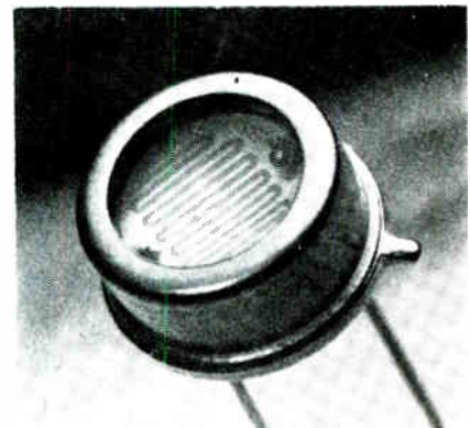
Eye for ultraviolet. Incident light can raise cell resistance a thousand fold.
