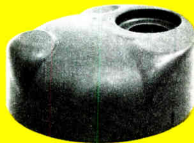
Stainless Steel 302; 7" diameter, .020" blank One draw • 10,000 psi
