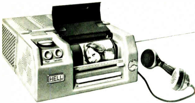
New for newsmen. Portable facsimile transmitter helps press photographers meet deadlines by speeding pictures back to their editors.
