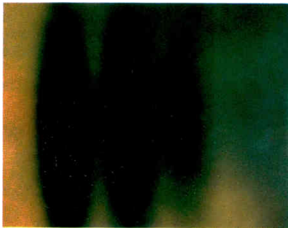
Scattering rod. Polaroid film depicts the electric field scattered by a metal cylinder 17 millimeters in diameter.
