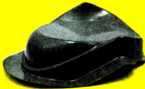
Aluminum 5257-0; 12" diameter, .035" blank One draw • 5,000 psi
