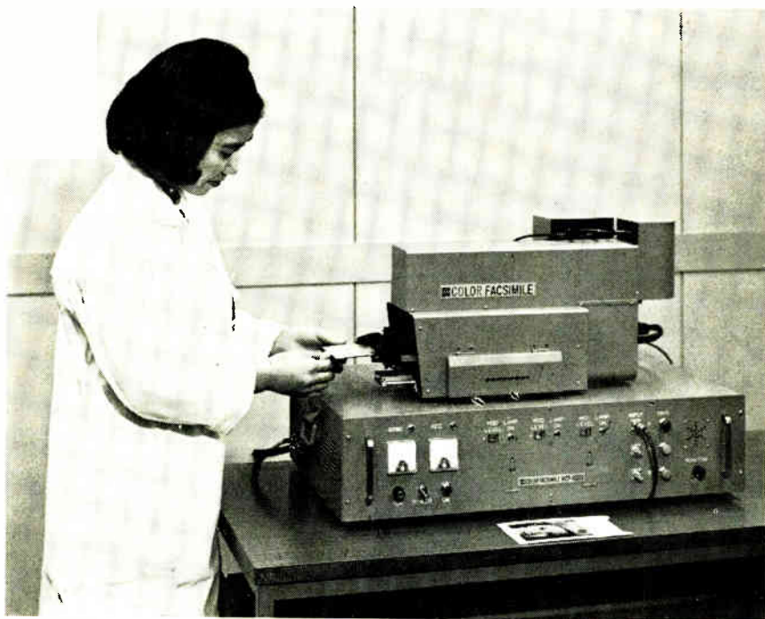
Fast and faithful. Primary colors transmitted simultaneously—and corrected individually—expose Polaroid film with high fidelity during 3.6-minute scan.
