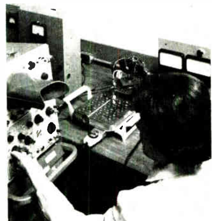
Checking. Operator checks SCR for turn-on characteristics to insure high di/dt .
