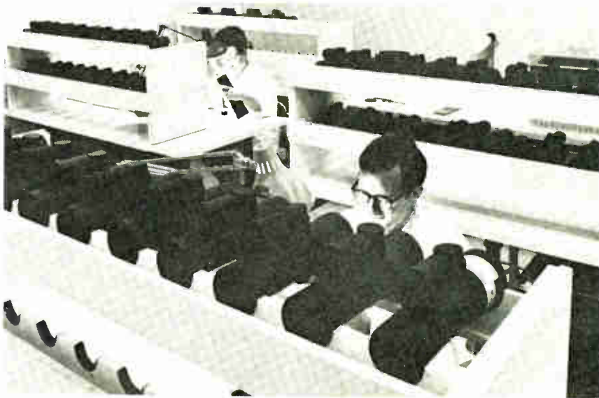
On the line. Technicians assemble Starlight night-vision scopes for the Army at Electro-Optical Systems in California.
