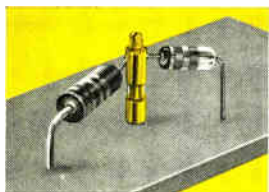
Solder one end to P/C board and attach lead to other end.
