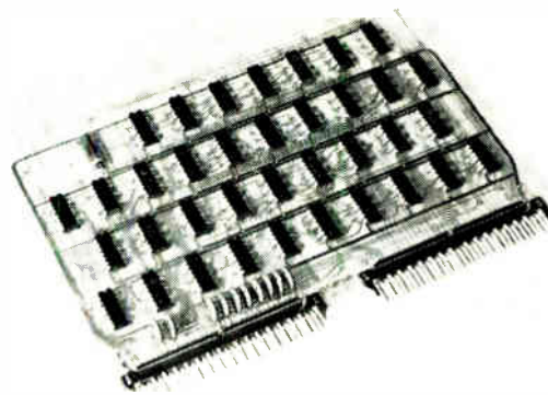
Five on one. Printed-circuit card contains functions for linearizing five transducers. Some portions of the circuits are shared, reducing cost per function.
