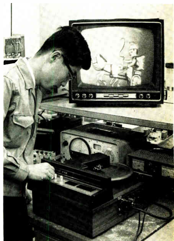
Video plateau. Television signals stored on record-like sheet of magnetic material can be played back instantly—fast or slow.
