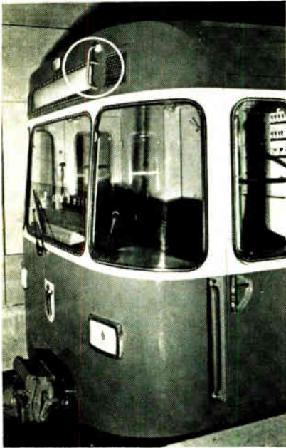
Inside or out. Quarter-wave antenna loop on Munich subway car works equally well in a tunnel or above ground.
