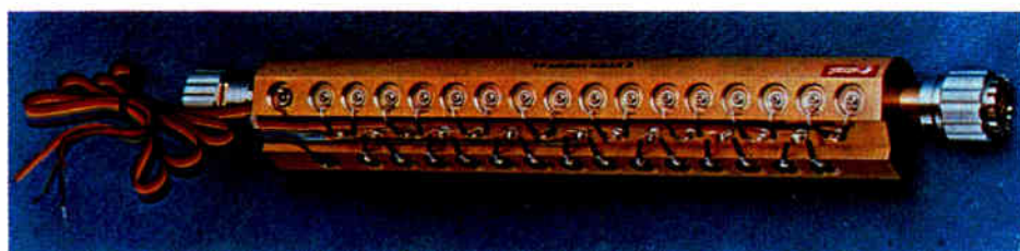
C-band shifter. By using 15 pairs of p-i-n diodes as switches, the device can introduce phase shifts in 22.5^\circ steps up to 337.5^\circ .
