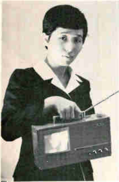
Svelte. Toshiba now has a prototype flat cathode-ray tube and may be first on the market with a book-size television set.
