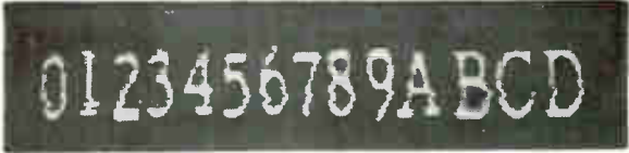
Number pick-up. Linear array of 40 phototransistors acts as a one-dimensional scanner for image sensor. To generate the second dimension, as shown by the number display, image is moved under the scanner.
