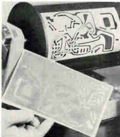
Dry copy. The finished p-c board requires no rinsing or cleaning.
