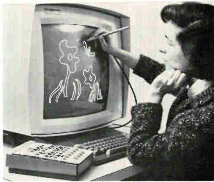
Textile designer uses computer-stored weaves, concentrates on designing novel patterns with light-pen input.
