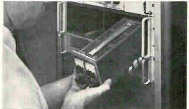
You can mount up to 4 units in a standard LRA-1 or LRA-2 rack adapter.
