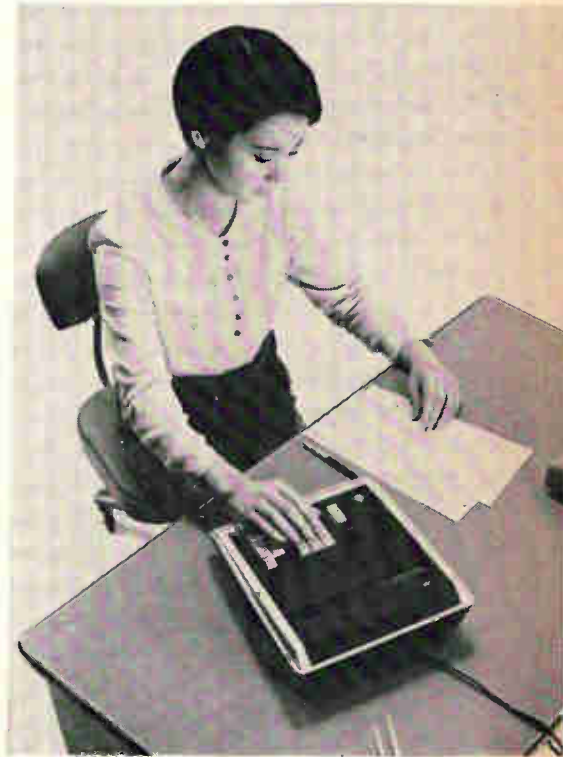
Calculating. Hayakawa Electric Co. plans to put desk calculator with metal-oxide-semiconductor logic circuits on the market late this summer. The company had prototypes on its stand at the IEEE convention.
