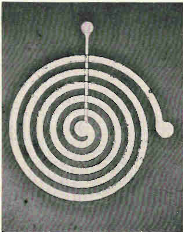
Lumped inductor is part of the lumped-element amplifier. It's outside diameter is 0.040 inch.
