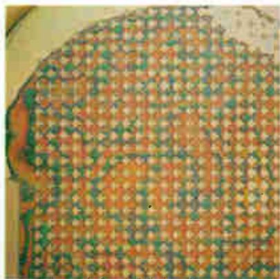
Close shave of wafer yields isolated transistor collector regions whose depths vary less than \pm 0.3 microns. Color fringes confirm accuracy.
