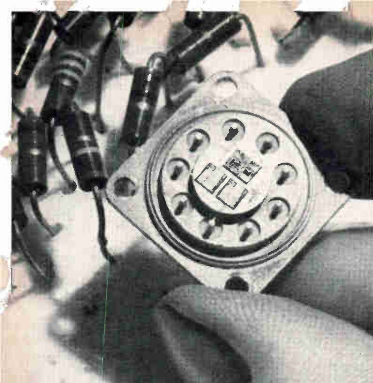
Forty-watt amplifier on three integrated circuit chips was designed with the aid of a computer by Norden division of United Aircraft Corp., Norwalk, Conn.
