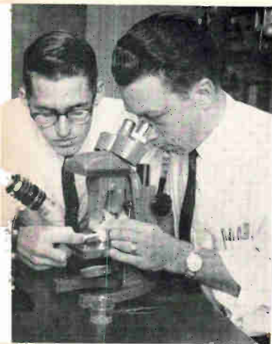
LSA mode. John Copeland, left, and Robert Spiwak, Bell Laboratories engineers, load a bulk n-GaAs diode into a 90-gigahertz oscillator circuit. Copeland will discuss the device, which operates in the LSA mode, at the Solid-State Conference.
