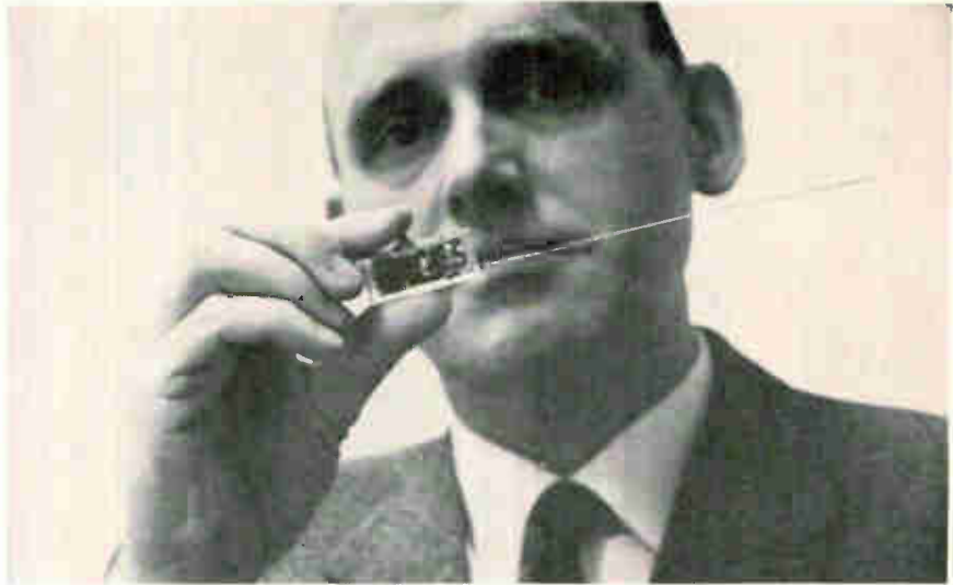
Calling all cars. Swedish police are testing a tiny prototype transmitter that officers could use to call for help. Svenska Radio AB developed the transmitter, which has thin-film circuitry.
