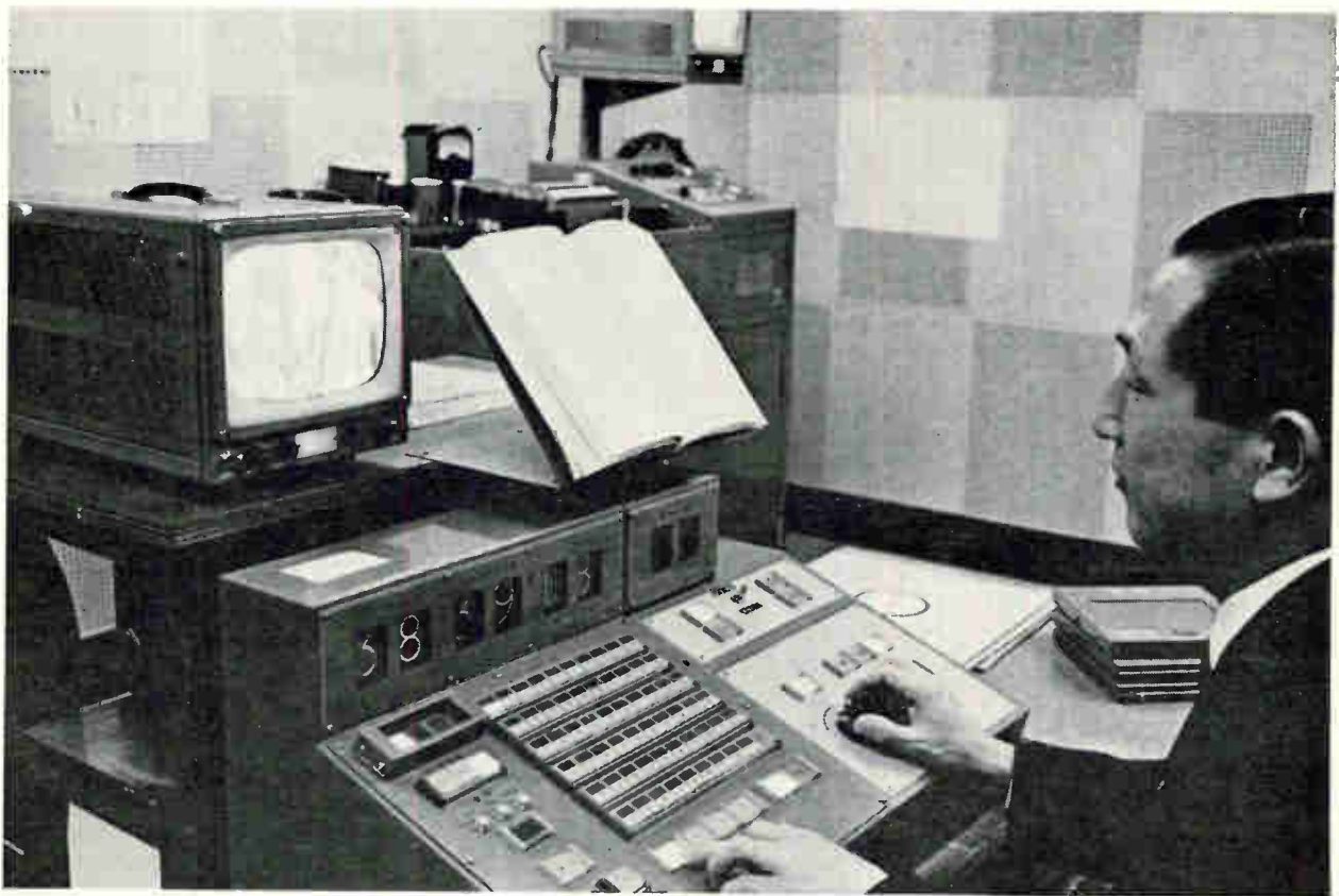
Television program director, at editing console, views monitor and selects scenes by push-button input to a process-control computer.
