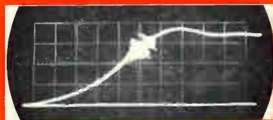
D Five minutes later, no significant drift; bird's marker is 100 Hz wide.
