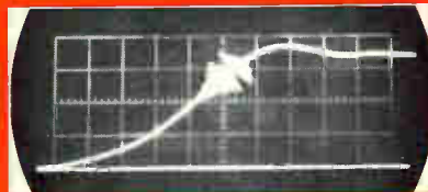
C. Same crystal filter as in (B) above, with 1/20 the sweep width (100 Hz drift).
