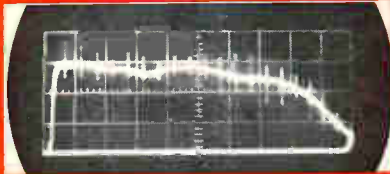
A. Frequency response of broad-band video amplifier, 100 kHz to 20 MHz.
