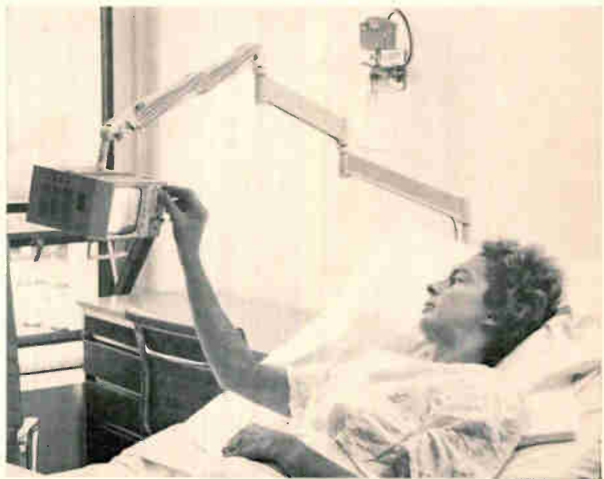
Patient can easily move and tune the 5½-pound receiver, which is supported by a gravity-free arm attached to the bed.
