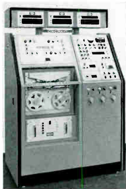
Acramatic IV numerical control is housed in this jukebox sized enclosure.
