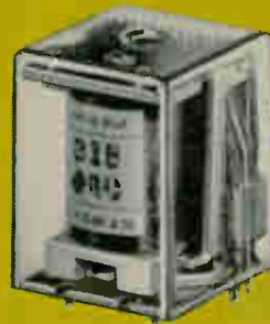
Type LB Relay has tinned nickel silver terminals for direct PCB mounting. Volume: 1.33 cubic inches. Maximum mounted height, 1.24 inches. Relay shown actual size.
