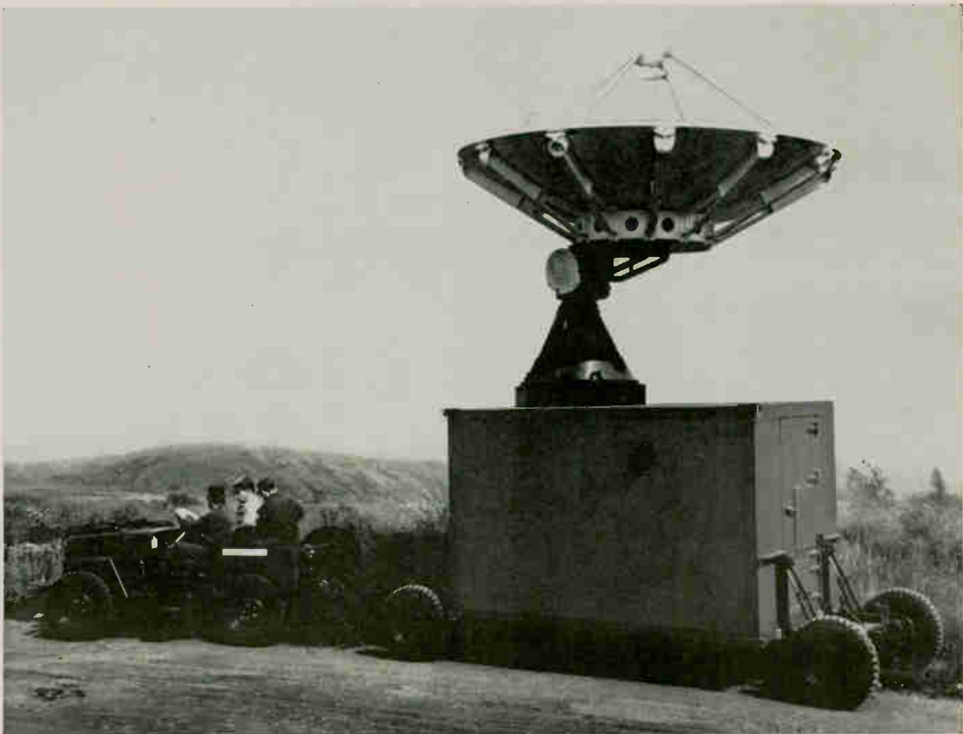
Sylvania's satellite communication terminal is one of the most mobile ground stations ever built. Weighing only two tons, it is readily transported by truck or helicopter. Three men can set it up in less than an hour. When used with Syncom III, this terminal provides one duplex voice channel and 16 simultaneous teletype channels.
