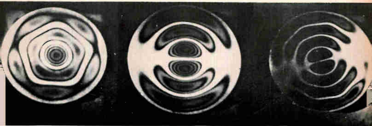
The series of light and dark lines on the reconstructed image indicate contours of constant vibrational amplitude.
