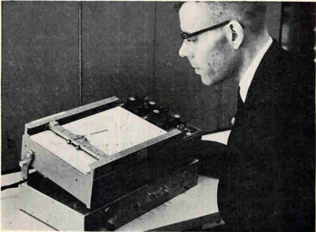
John Gersbach inspects a shmoo curve drawn by his automatic device. The circuitry of the plotter is entirely in the chassis at bottom; the x-y recorder is a commercial unit connected to the plotter. If an actual test were under way, wires would be connected to terminals at the far end of the plotter.
