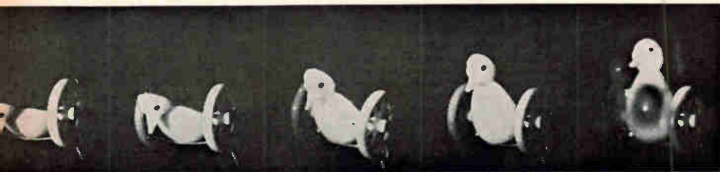
Movie made by recording five frames holographically on a thick emulsion. The photographic plate was rotated slightly between exposures to store the successive pictures. The movie was read out by repeating the rotation while the plate was illuminated with the light beam.
