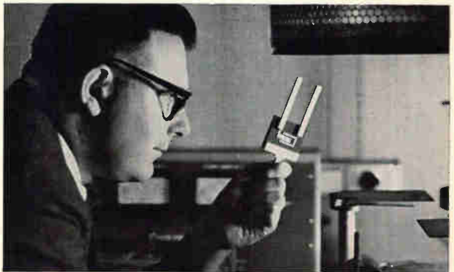
M. P. Lepselter examines beam-lead model (enlarged about 300 times). Beams were thermally aged in 360° C steam for 1000 hours, centrifuged to 130,000 G, bent 90° twenty times without failure. Beams can be tapered for smooth impedance matching, widened to act as heat sinks.
