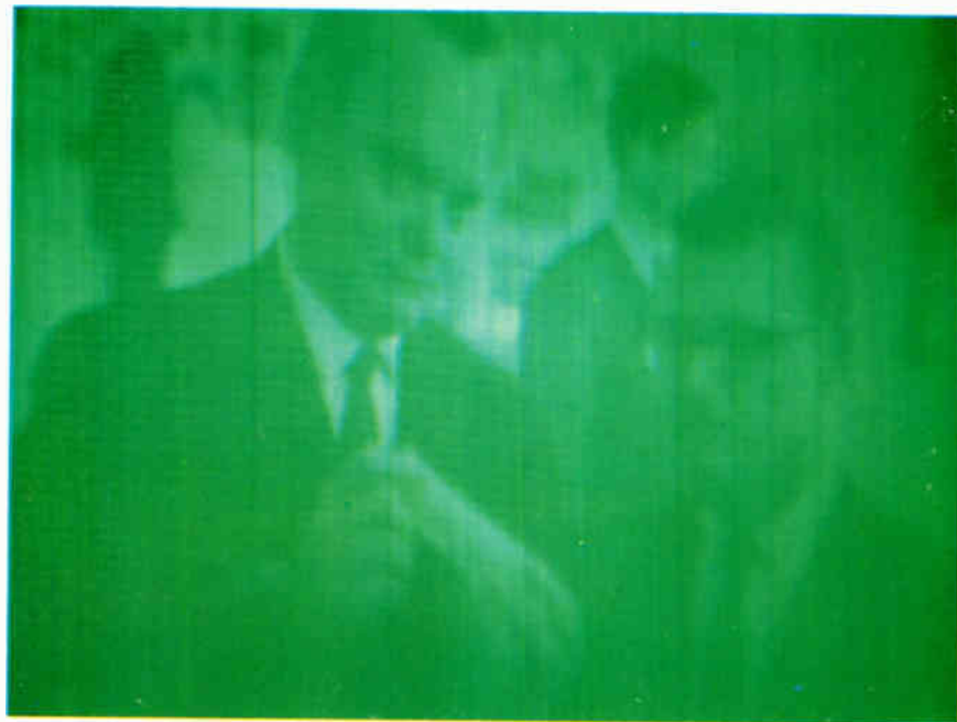
Laser display from Texas Instruments Incorporated projects blue and green beams. TI has a prototype system that adds red.
