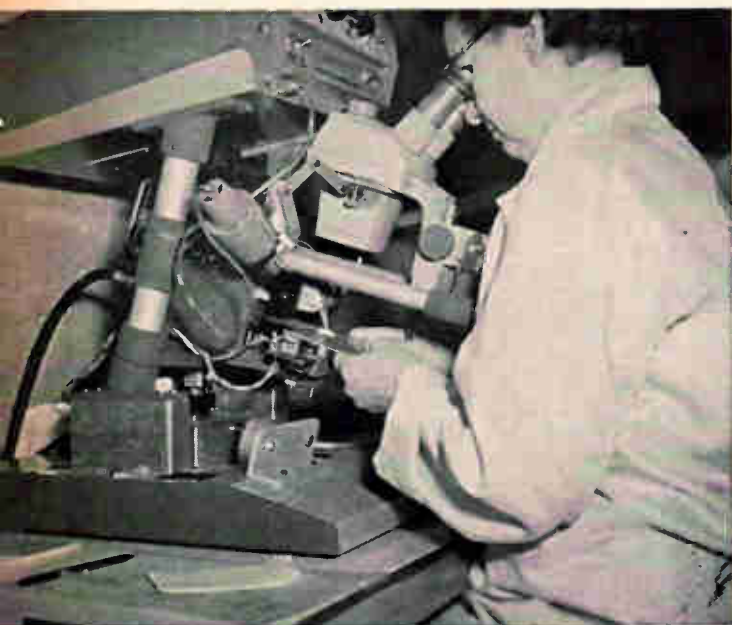
Parallel-gap welding with an automatic welding machine takes about 30 seconds per flatpack. The view at right is through operator's stereoscopic magnifiers. The configuration of the electrodes gives the technique its name.
