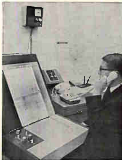
Printer-recorder in dispatching center of Hamburg bus company shows where each bus on a route should be and where it actually is.
