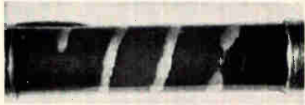
Example of carbon film resistor with conducting bridge detected by the nonlinearity method. Where the dark resistive film crosses the ground spiral gap of the resistor (light area) current flow causes the nonlinearity.
