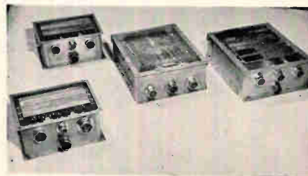
First equipment made with the avionics modules was this prototype of a random-access telemeter, consisting of 51 modules and four matrixes, housed in four boxes.
