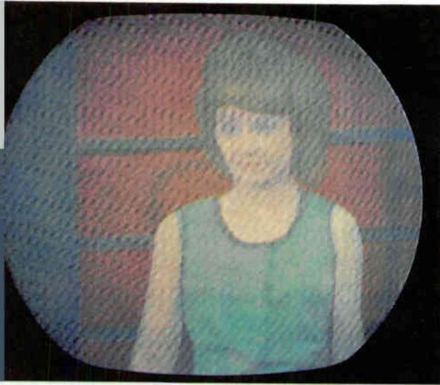
Cross-modulation components that are 43 db below signal level produce noticeable interference.
