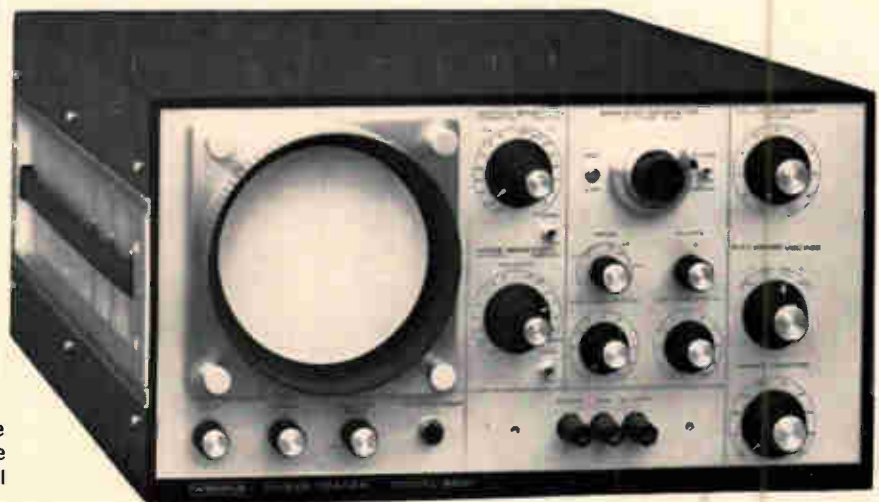
Calibrated controls beside curve-tracer screen provide unambiguous readout of vertical and horizontal sensitivity.
