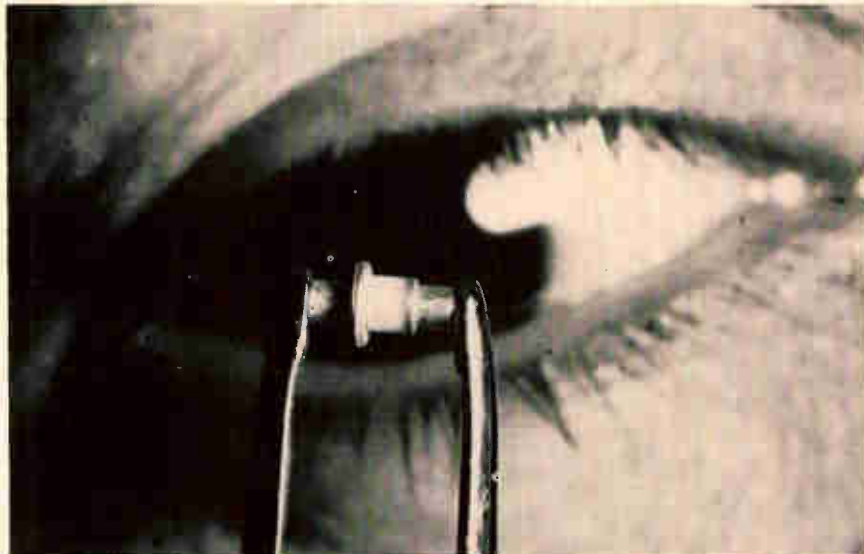
Gallium-arsenide diode is mounted in a metal-ceramic package; the pn junction oscillator can do the work of a low-power klystron tube 50 times as heavy.
