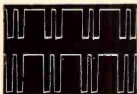
Attenuator Characteristics Upper trace: 30mv Lower trace: 10V
