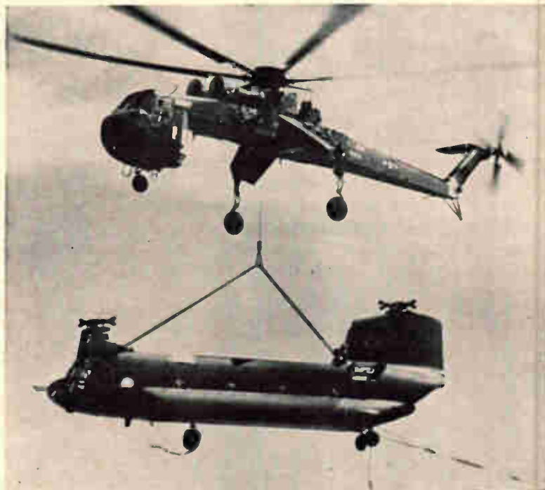
Damaged by Viet Cong fire, a Chinook helicopter gets a lift from a Skycrane back to a military base for repairs. Production of both craft will be stepped up for the military.
