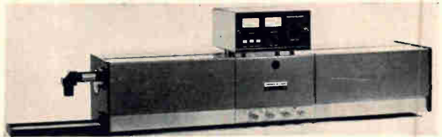
Molecular gas laser with continuous-wave infrared output has a variety of potential applications, including welding, surgery and communications.
