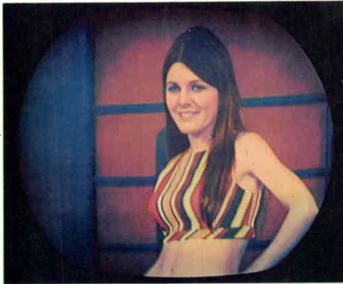
Good pictures are received when cross-modulation and noise are 48 db or more below the signal level.
