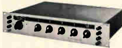
Figure 2. Resolver/Synchro Simulator provides ideal source for receiver testing.
