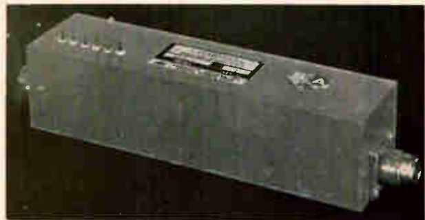
Ferrite phase shifter with reciprocal and latching properties is switched in 22\frac{1}{2}^\circ increments by low-power pulses.
