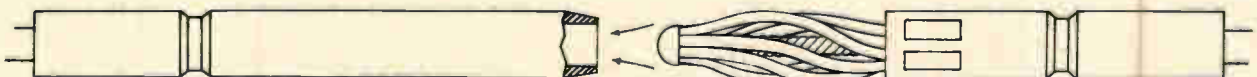
Strands, carefully twisted, form counterwound helices to give connector pin added rigidity and reliability.
