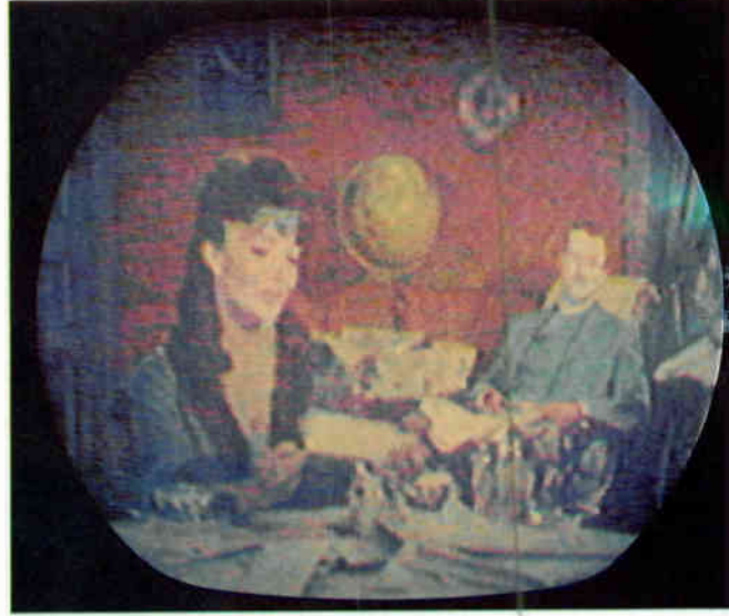
Noise randomly triggers color circuitry, causing confetti-like pattern on the television screen.
