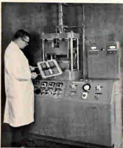
This 25-ton 359D packaged system includes molds, loading frames, and controls for economical, direct encapsulation by transfer molding.
