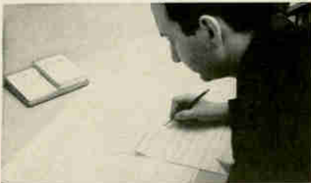
Trial arrangement of IC packages is made on a component layout master to provide an interconnection schedule.
