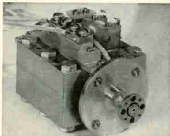
Traveling-wave maser has a superconducting field coil that is housed in the metal section attached to the left side of the maser.
