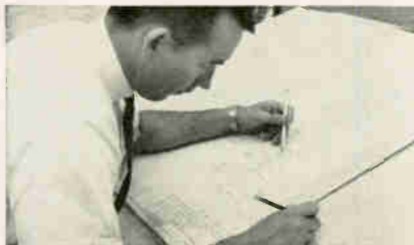
Wiring layouts on board-artwork masters are checked against the logic diagram.
