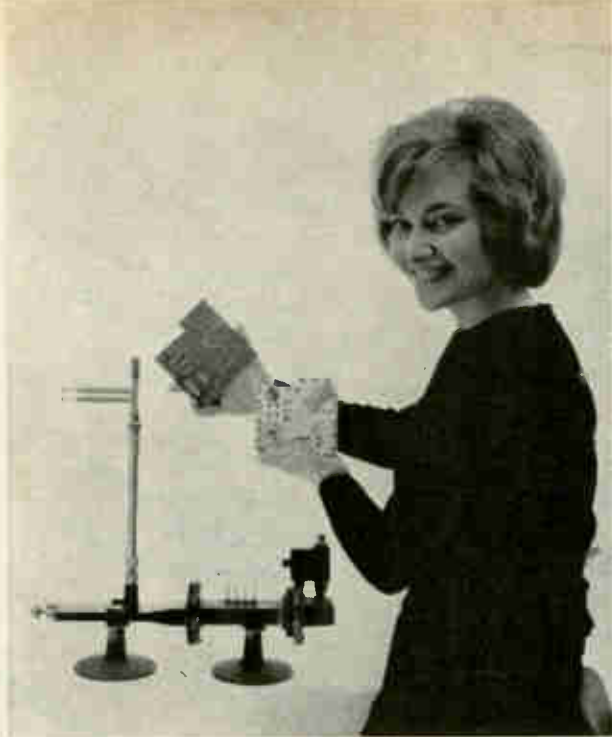
Comparison of equivalent microwave and strip transmission line circuits shows the reduction in size offered by the latter technique. Girl holds both the basic strip transmission line circuit board and the complete package for a varactor tripler.
