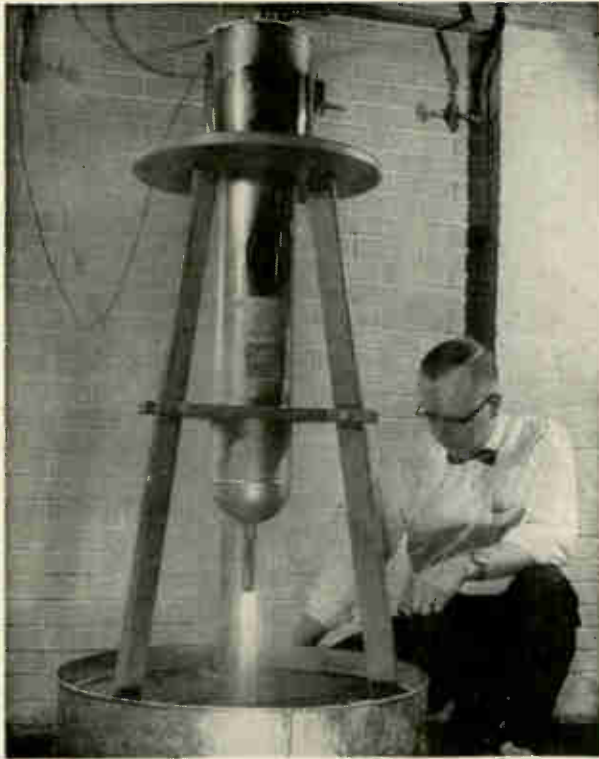
Magnetohydrodynamic (MHD) generator uses a 1-inch air-core superconducting coil for the field coil. The coil and its support are being lowered into the Dewar vessel.
