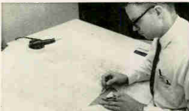
Signal-wiring layout is prepared on vellum over the logic design master pattern.
