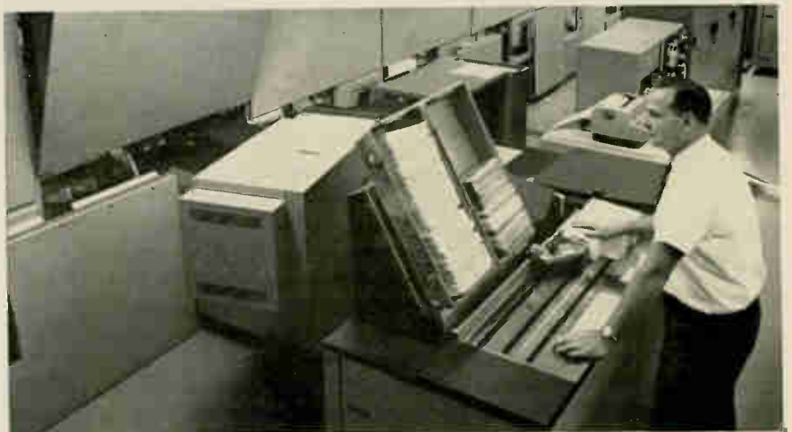
Optical scanner developed by the Philco Corp. can sort 30,000 pieces of mail an hour. The Post Office Department will soon order nearly $100 million of equipment to automate its operations.
