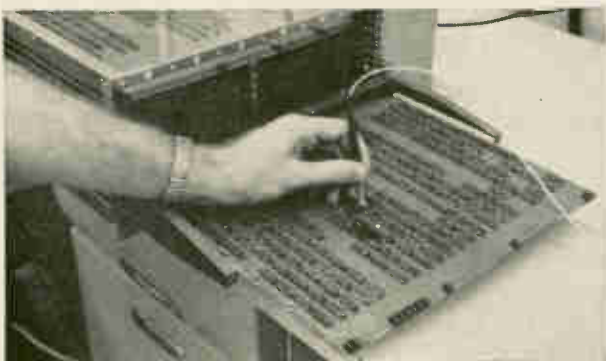
After system fabrication, card extenders expose the boards for functional testing and debugging.
