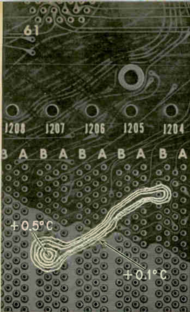
Thermal profile showing hot spot (temperature rise to 0.5° C) is superimposed on photo of a portion of a multilayer board. The system usually prints out hot-spot locations, rather than preparing profiles.
