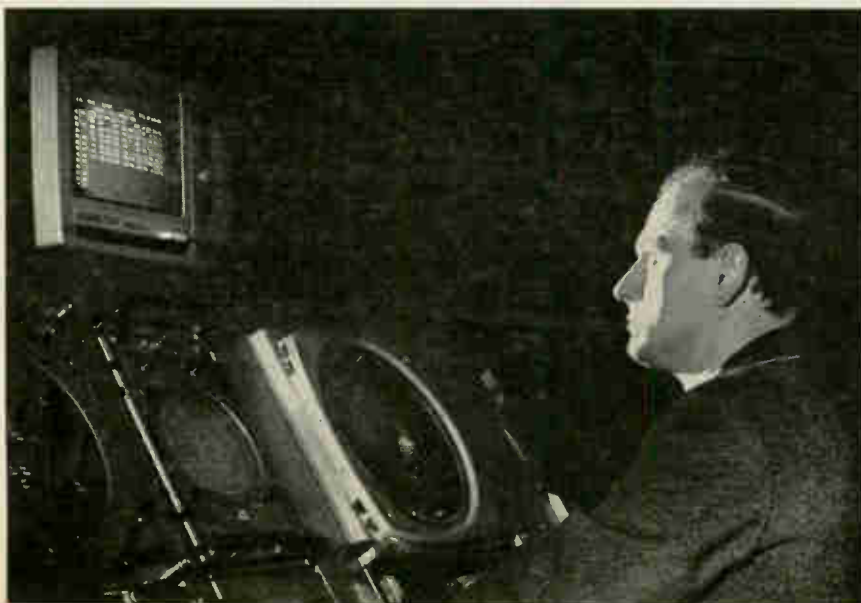
Flexible data presentation, made by Marconi Co., being tested at Prestwick, Scotland. Display at top shows flight-progress data relating to display at right. Radar display at left shows only digitized data derived from the original radar-video signal.
