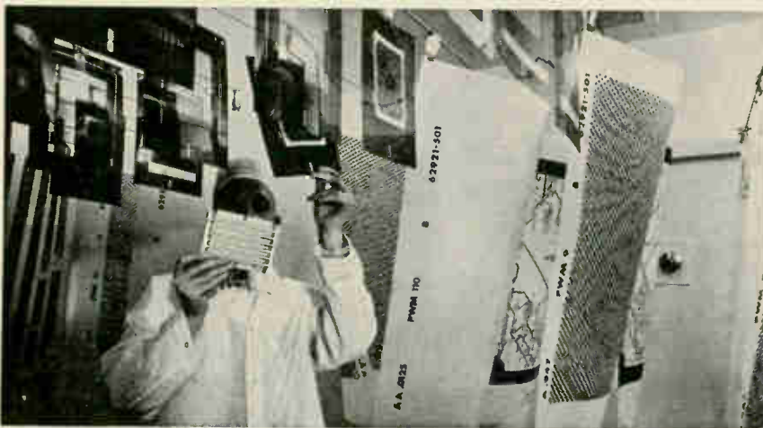
Large negatives, hanging up to dry after photographic processing, are reduced to size of tool film held by lab technician.
