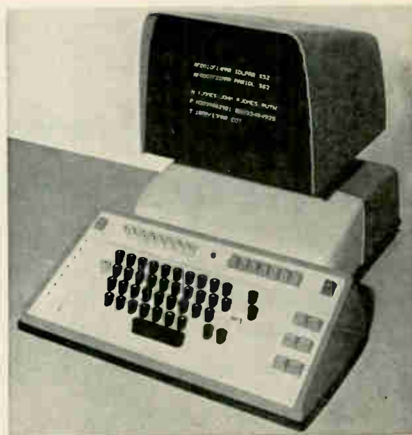
Cathode-ray tube display of the type used in the time-shared computer system at the University of Pennsylvania. The keyboard includes function and editing keys for message composition and correction. The unit is a Bunker-Ramo model 203 display station.
