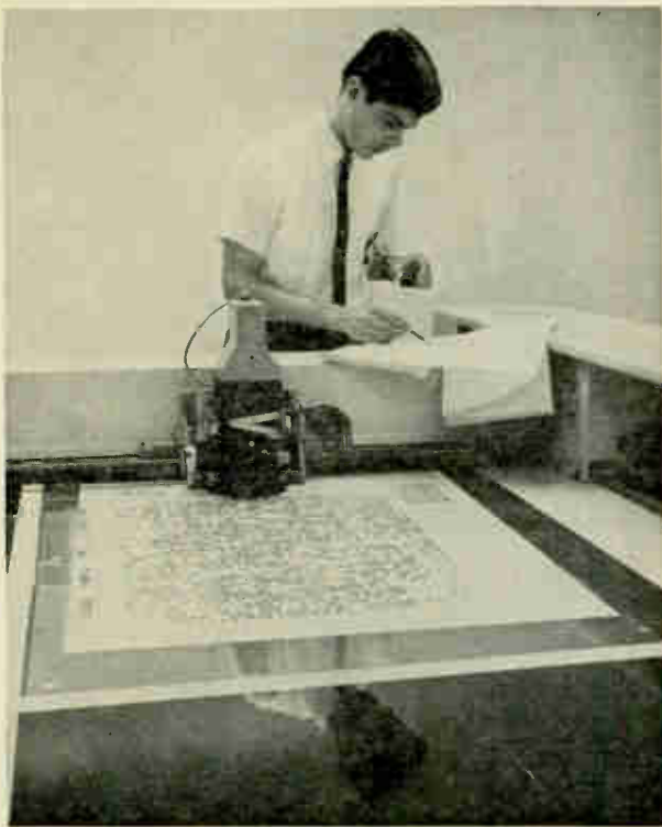
Master negative for a board layer is prepared automatically with this computer-programed drafting machine. Standard parts of the pattern, such as pads and line segments, are generated photographically.
