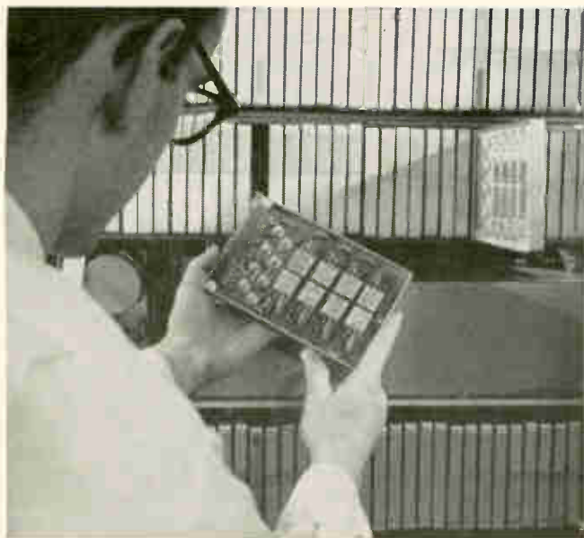
Experimental automatic data equalizer devised at Bell Laboratories. Control section consists of the circuit packages; the package being inspected is one of 12 attenuators, the settings of which determine the degree of distortion-correction of the equalizer.
