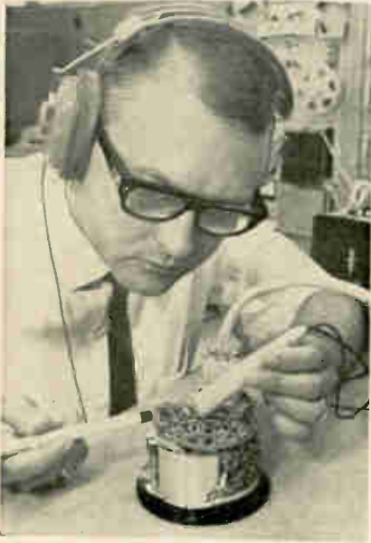
Listening for r-f noise in a micro-electronic assembly is Richard T. Stevens, senior systems development engineer at Honeywell.
