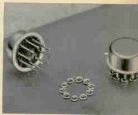
In a typical application, transistor cans are made pluggable to boards by inserting and flow soldering AMP's miniature spring contacts
