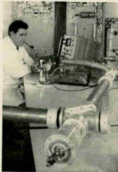
Experimental waveguide being tested at CGE research center in Marcoussis.
