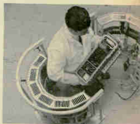
AMP's subminiature printed circuit connectors conserve space in missile guidance and control computer
