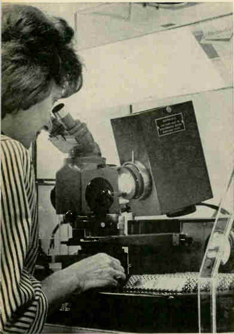
Operator aligns working plate with silicon wafer for exposure of photoresist with ultraviolet source.
