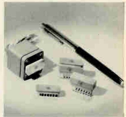
Production test socket (left) and breadboarding sockets (right) are being developed for plug-in flat packs.
